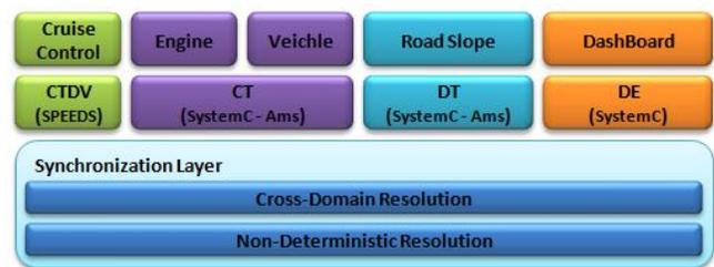
Figure 4 - DESYREII / DESYREML Layered Architecture
