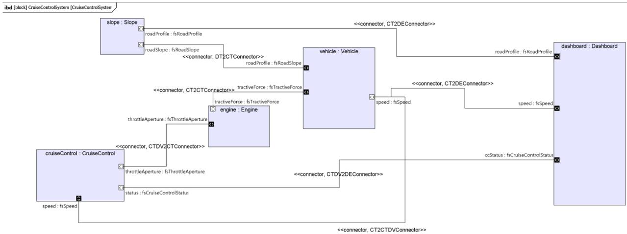
**Figure 2 – Cruise Control Internal Block Diagram**
