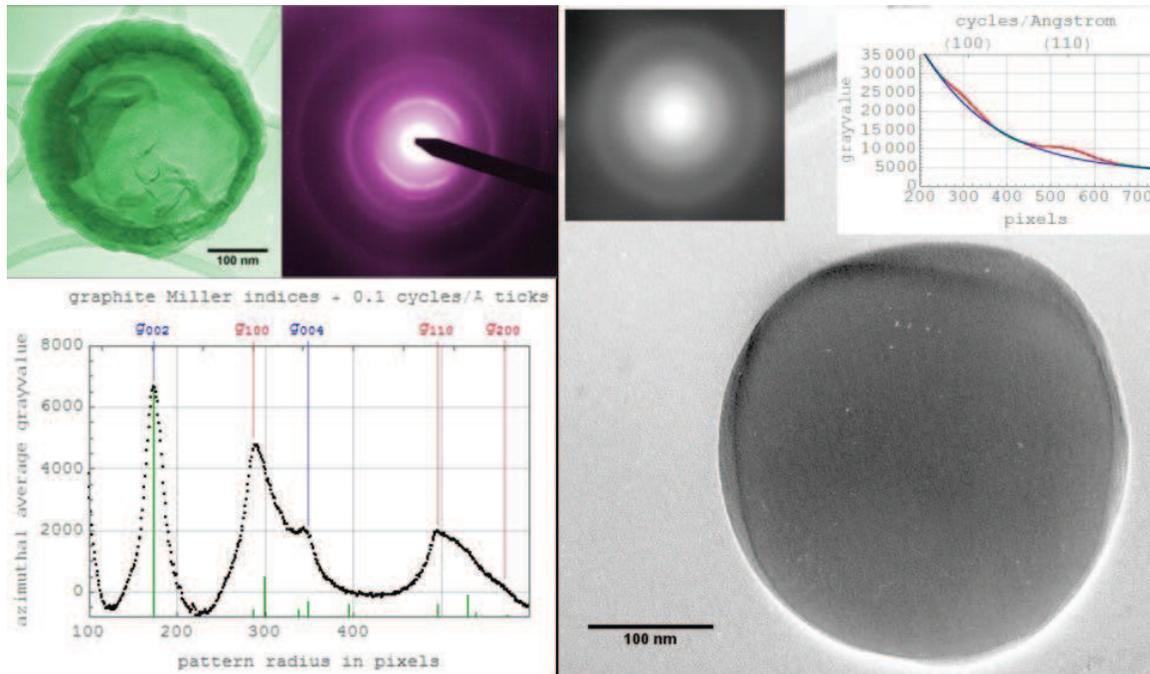
**Figure 3.** Left half - Brightfield TEM image at top of a graphite particle from our third annealing run, a selected area diffraction pattern of the whole particle at top right, and a background subtracted azimuthally-averaged profile analysis at bottom; Right half - at top left a selected area diffraction pattern of the core-only particle shown at bottom, and an azimuthally-averaged profile showing broad graphene-only peaks.
