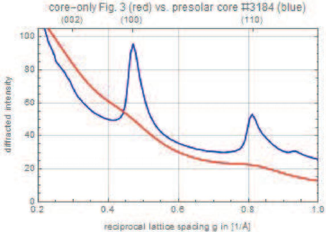
**Figure 5.** Comparing diffraction profiles of the “homemade” core-only particle profiled on the right side of Fig. 3, with the diffraction profile from the core-region of a presolar core-rim particle (Mandell et al. 2006), to show that the size and abundance of un-layered graphene sheets in the “homemade particles” is still much smaller than those found in the presolar cores.
