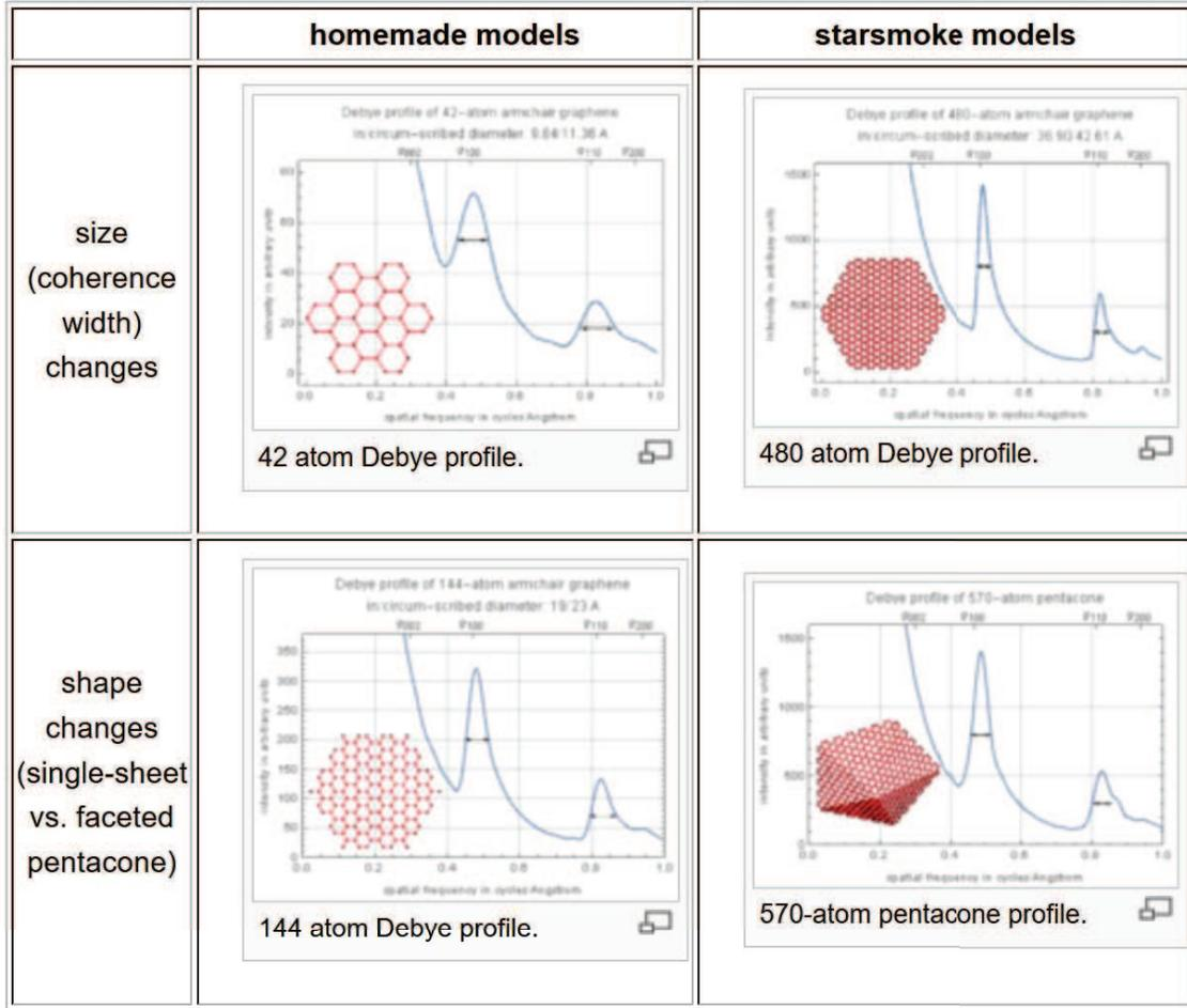
**Figure 6.** This comparison of graphite sheet size and shape effects on the “Debye scattering equation” diffraction profile average over all orientations (Warren 1969) were first applied to this problem by Mandell (2007).
