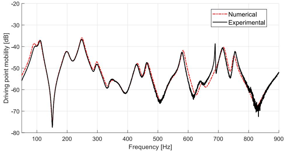
Figure 6: Experimental and numerical comparison of the frequency response functions of the panel with piezoelectric patches connected to a multi-resonant network.
