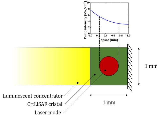
Fig. 2. Position of the laser mode in the 1 mm<sup>2</sup> section of the crystal. Inset, pump intensity distribution along the pump axis.
