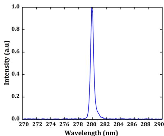
Fig. 8. Spectrum of the UV pulse after THG.
