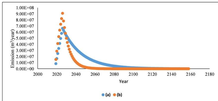
**Figure 2.** Estimate methane emission from Kossihouen landfill site from 2019 to 2160. (a): default values of  $K$  and  $L_0$  were be used to estimate methane emission; (b): determined values of  $K$  and  $L_0$  were be used to estimate methane emission.
