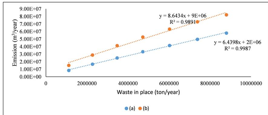
**Figure 3.** Annually increasing the methane production from disposed waste in landfill site from 2019 to 2025. (a): default values of  $K$  and  $L_0$  were be used to estimate methane emission; (b): determined values of  $K$  and  $L_0$  were be used to estimate methane emission.
