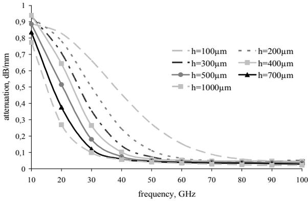
Fig.2: Attenuation (dB/mm) of the PGL versus the frequency (10-100GHz) for different thicknesses of Silicon and a strip width of 100µm
