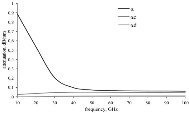
Fig.7 : Attenuation (dB/mm) of the PGL versus the frequency (10-100GHz) ( $t_{strip}=1\mu m$ ,  $h_{Silicon}=500\mu m$ ,  $w=100\mu m$ ) in considering total losses  $\alpha$ , metallic losses  $\alpha_c$  or dielectric losses  $\alpha_d$
