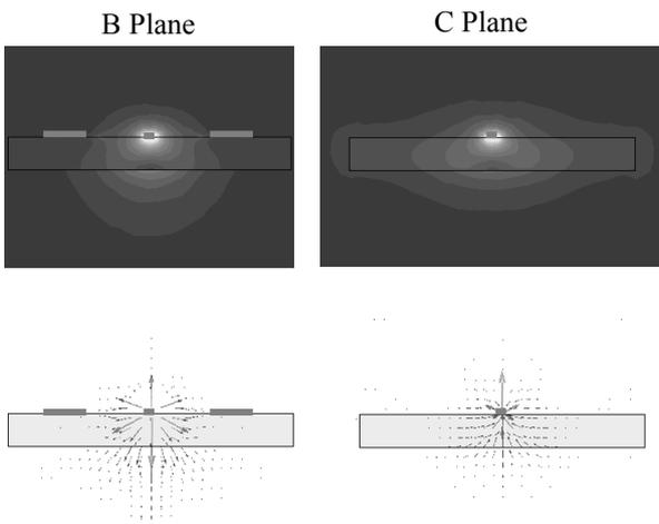
Fig.9: Cross-section E-field distributions along the coplanar-tapered PGL transition for  $h_{Silicon}=350\mu m$  (B Plane and C Plane of figure 1)
