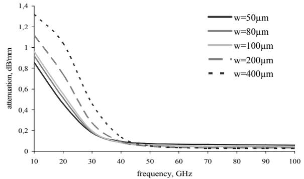
Fig.5: Attenuation (dB/mm) of the PGL versus the frequency (10-100GHz) for different strip widths ( $t_{strip}=1\mu m$ ,  $h_{Silicon}=500\mu m$ )
