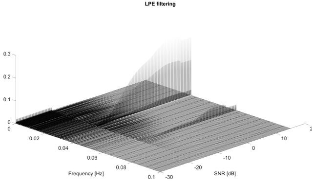
Figure 4: Squared envelope spectrum waterfall plot after filtering with the proposed method based on the relative prediction error.
