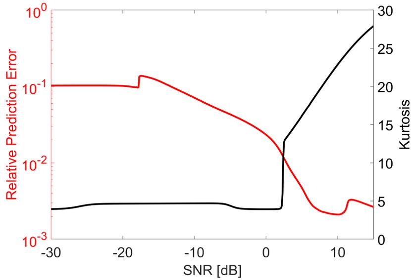
Figure 2: Trending of Relative Prediction Error (RPE) versus kurtosis after blind filtering using the proposed LPE approach and MED respectively.
