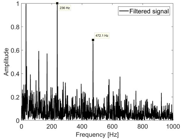
Figure 6: Experimental case: (Left) The envelope spectrum of the raw input signal. (Right) The envelope spectrum after filtering with the proposed LPE method.
