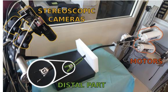
**Figure 2:** The experimental setup consists of the STRAS robotic platform and the external measurement system composed of two cameras and Chillitag markers [6].
