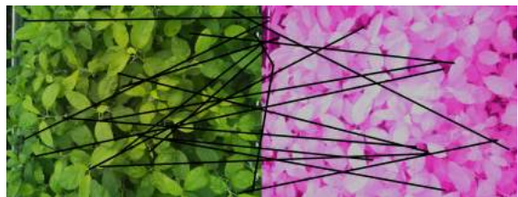
Figure 2: Keypoints found by SIFT and the 20 strongest matches on an image pair, drawn as black lines.
