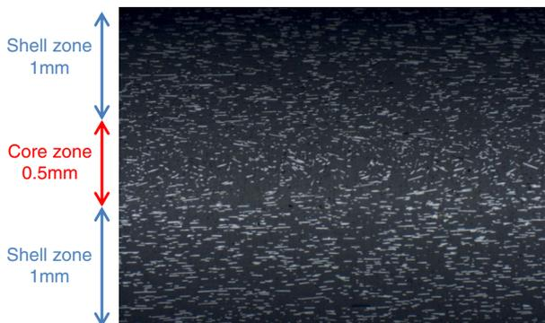
**Fig. 11** Microscopic observation of the composite PPr-CF180 structure
