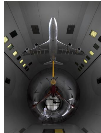
ONERA S1MA test section Diameter 8 meters Length 14 meters
