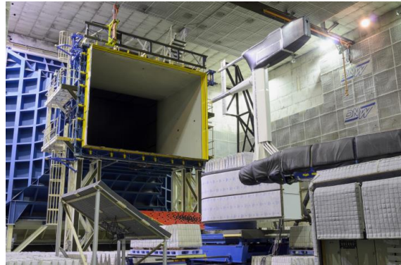
Acoustic calibration setup with installed loudspeaker noise source (provided and operated by Airbus).
