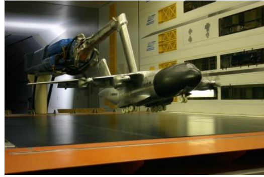
LLF test section 8 x 6 meters ground effect test setup
