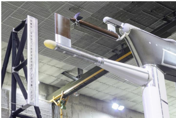
APIAN-INF propeller model with installed pylon.
