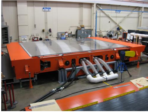
DNW moving belt during the factory acceptance test
