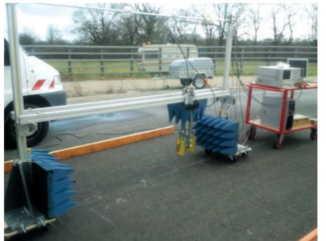
FIGURE 1. The French Research Institute of Science and Technology for Transport, Development, and Networks' (IFSTTAR's) air-coupled step-frequency GPR and the automated bench to scan the near subsurface [14].
