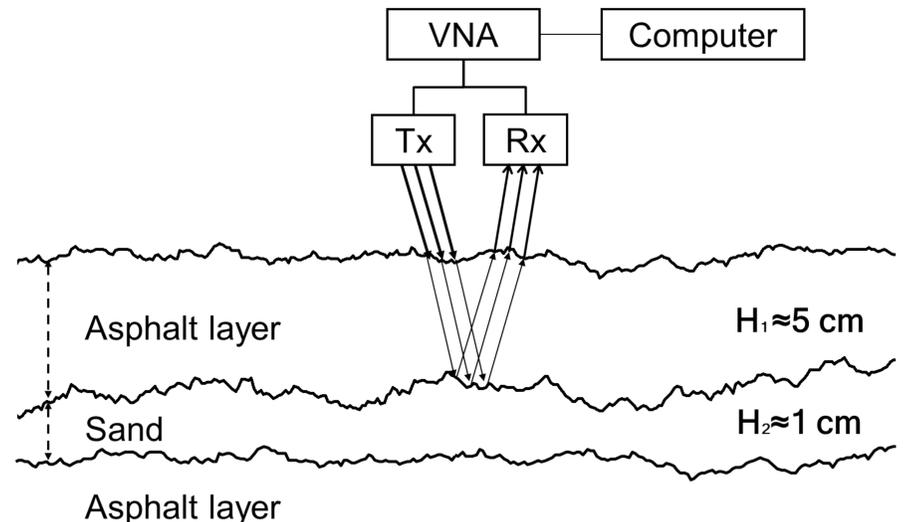
Figure 1: GPR and pavement configuration.
