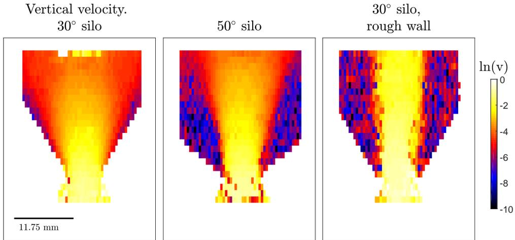
FIG. 3. The log of the magnitude of the vertical component of velocity ( $v$ ) is plotted for each of the three silos. Mass flow is observed in the  $30^\circ$  silo, funnel flow in the  $50^\circ$ , and rat-holing in the  $30^\circ$  silo with rough walls (with particles glued to the silo wall). Yellow regions indicate rapid flow, while purple/blue areas indicate slow to stagnant zones.
