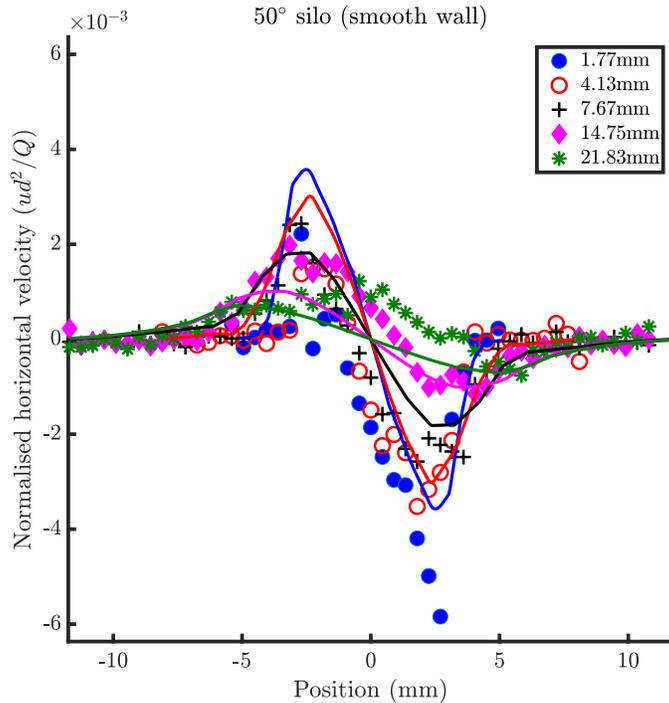
FIG. 10. The horizontal velocity MRI measurements (solid circles) compared with those predicted by the numerical model (lines) for the  $50^\circ$  silo. at the same locations as in the vertical velocity figure.
