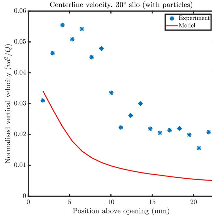
FIG. 13. A comparison of the normalised vertical velocity measured along the axial centerline of the silo compared with that predicted by the model for the  $30^\circ$  silo with roughened walls.
