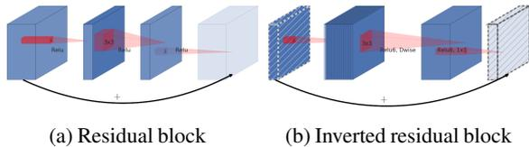
Figure 3: MobileNetV2 uses inverted residual blocks to reduce the number of channels that are forwarded in subsequent layers. Figure from [23].
