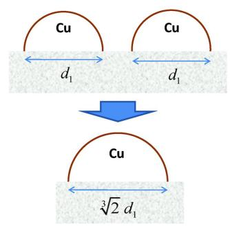
15 Fig. 7 (Color online) Schematic model showing the result of coalescence of two identical hemispheric Cu particles, with conservation of the total volume of Cu and the hemispherical morphology.
