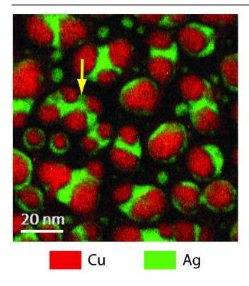
**Fig. 3** (Color online) Superimposed Ag and Cu elemental map of sample 2@1-100 obtained by EFTEM using the three-window technique. The 5 arrow designs a CuAg ensemble with six copper cores linked by silver.
