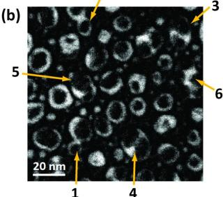
**Fig. 2** (Color online) (a) Zero-loss EFTEM image on a representative area <sup>20</sup> of sample 2@1 and (b) Ag elemental map obtained by Energy Filtered TEM on the same area.
