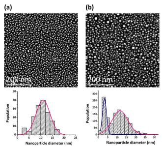
**Fig. 1** (Color online) HAADF-STEM images of samples (a) 2@0 Cu and (b) 2@1 CuAg. The size distribution for each micrograph is also <sup>90</sup> presented. Characteristics of the distribution are detailed in Table 1.
