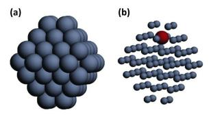
**Fig. 8** (Color online) Model for the truncated octahedral  $Ag_{78}Cu_1$  cluster <sup>20</sup> used in the DFT, P1 and P2 calculations. The external surface of the  $Ag_{78}Cu_1$  cluster is represented in (a). The cluster configuration in (b) represent the Cu atom in the most favorable place according to DFT calculations.
