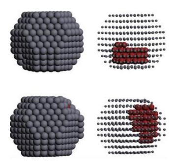
35 Fig. 9 (Color Online) Structure of a truncated octahedron of 586 containing 90% Ag and 10% Cu after global optimization runs of exchange moves only. The structure is somewhat distorted to release the strain. In the top and bottom row we show the results of P1 and P2, respectively. In both models, quasi-janus configurations are obtained.
