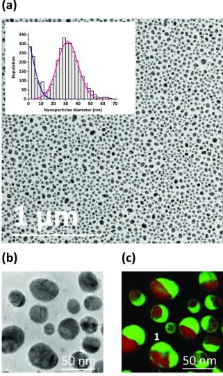
**Fig. 6** (Color online) Annealing experiment on 2@1-100 sample. (a) Bright field TEM image of the final configuration of the bimetallic <sup>55</sup> nanoparticles. The inset shows the size distribution of the particles. (b) Zero-loss EFTEM image on a representative area of sample 2@1-100 sample and (c) superimposed Ag and Cu elemental map of sample 2@1-100 obtained by EFTEM using the three-window technique on the same area. Color code identical to Fig. 3.<sup>12,13</sup>
