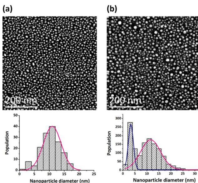
**Fig. 1** (Color online) HAADF-STEM images of samples (a) 2@0 Cu and (b) 2@1 CuAg. The size distribution for each micrograph is also presented. Characteristics of the distribution are detailed in Table 1.
