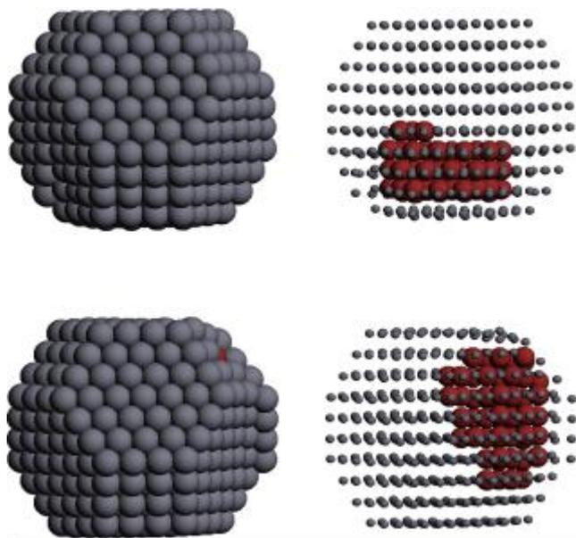
**Fig. 9** (Color Online) Structure of a truncated octahedron of 586 containing 90% Ag and 10% Cu after global optimization runs of exchange moves only. The structure is somewhat distorted to release the strain. In the top and bottom row we show the results of P1 and P2, respectively. In both models, quasi-janus configurations are obtained.
