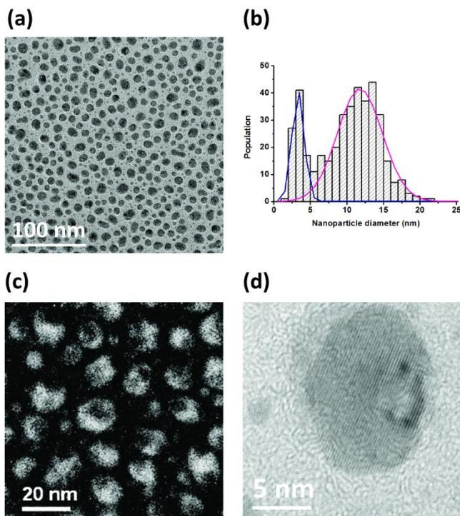
**Fig. 4** (Color online) TEM observations of sample 1@2. (a) Bright field TEM image on a representative area of the sample, (b) the size distribution of sample 1@2, (c) Ag elemental map obtained by EFTEM using the three-window technique and (d) HRTEM image of a Janus nanoparticle.
