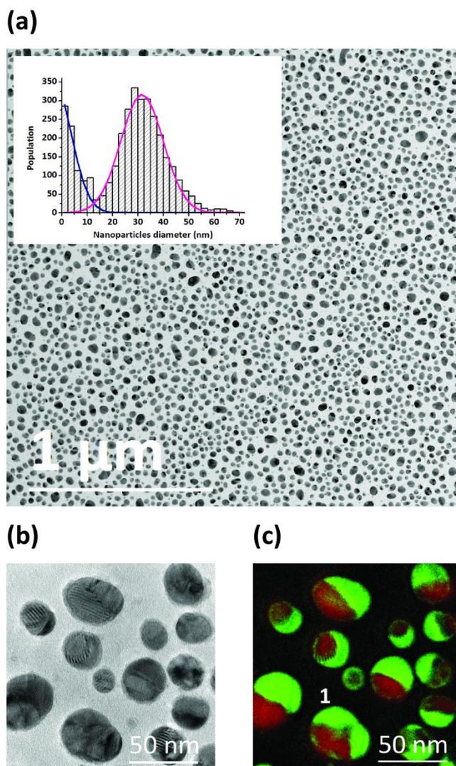
**Fig. 6** (Color online) Annealing experiment on 2@1-100 sample. (a) Bright field TEM image of the final configuration of the bimetallic nanoparticles. The inset shows the size distribution of the particles. (b) Zero-loss EFTEM image on a representative area of sample 2@1-100 sample and (c) superimposed Ag and Cu elemental map of sample 2@1-100 obtained by EFTEM using the three-window technique on the same area. Color code identical to Fig. 3.<sup>12,13</sup>
