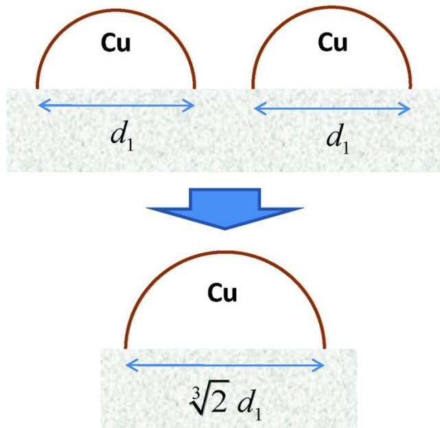
**Fig. 7** (Color online) Schematic model showing the result of coalescence of two identical hemispheric Cu particles, with conservation of the total volume of Cu and the hemispherical morphology.
