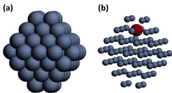
**Fig. 8** (Color online) Model for the truncated octahedral  $\text{Ag}_{78}\text{Cu}_1$  cluster used in the DFT, P1 and P2 calculations. The external surface of the  $\text{Ag}_{78}\text{Cu}_1$  cluster is represented in (a). The cluster configuration in (b) represent the Cu atom in the most favorable place according to DFT calculations.
