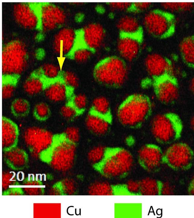
**Fig. 3** (Color online) Superimposed Ag and Cu elemental map of sample 2@1-100 obtained by EFTEM using the three-window technique. The arrow designs a CuAg ensemble with six copper cores linked by silver.
