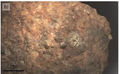
Fig. 6. Photographs illustrating the alteration crusts covering the pigment on samples (a) DPK15-5 and (b) DPK15-06
