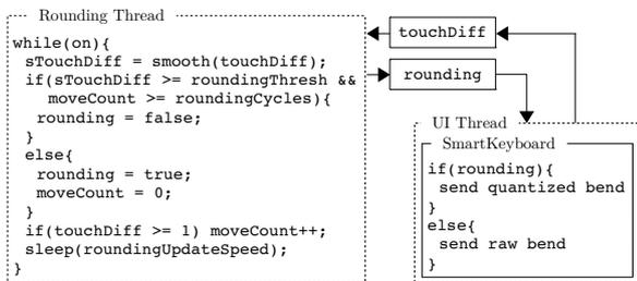
Figure 3: SMARTKEYBOARD pitch rounding pseudo code algorithm.
