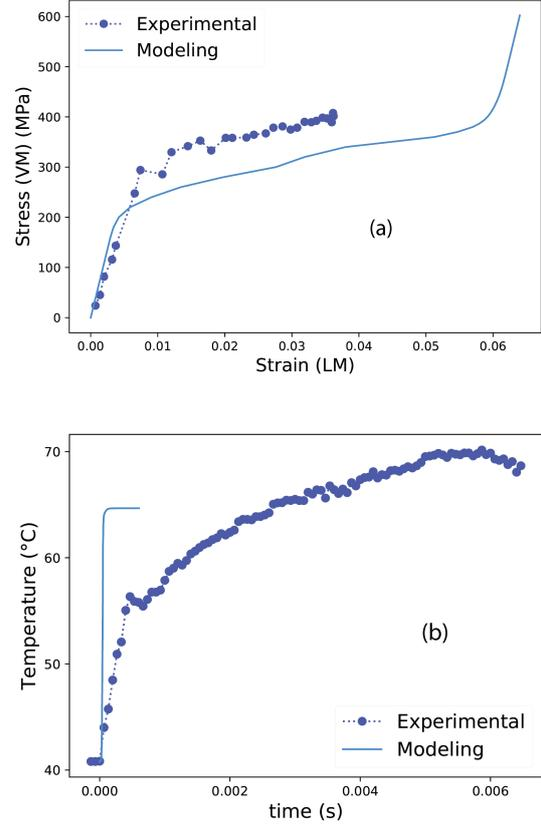
Figure 7: Comparison experiments modeling: (a) Normalized stress-strain behavior; (b) Temperature release.
