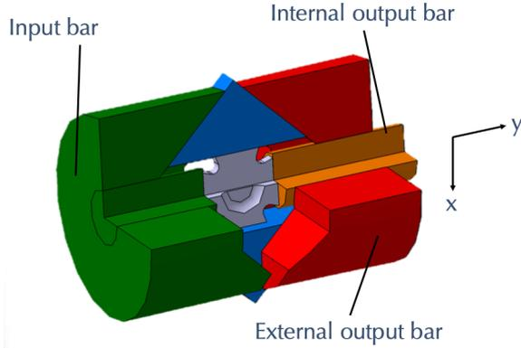
Figure 1: Set-up principle for dynamic equibiaxial compression test.
