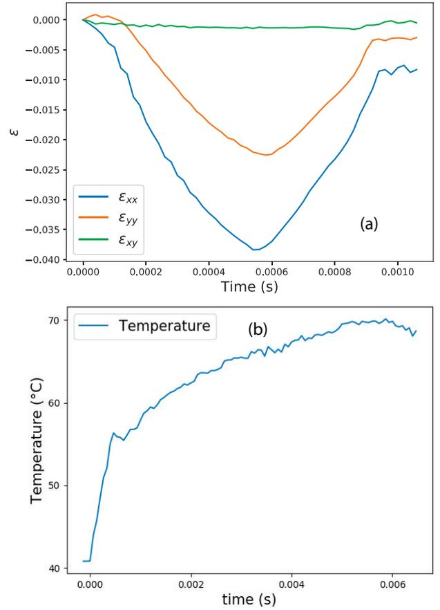
Figure 4: Average strain components and temperature over the ROI from DIC and infrared observations
