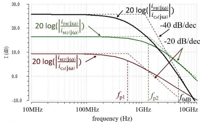
Fig. 9. Cadence™ simulation of the two-step current mirror transfer function ( $i_{\text{bias}} = 2\text{mA}$ ,  $dv/dt = 6\text{V/ns}$ ,  $G = 20$ , CMOS  $0.18\mu\text{m}$  technology).
