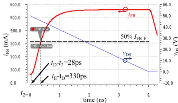
Fig. 7. Simulation of the transient response time with  $G = 20$  ( $v_{DRV} = 4V$ ,  $i_{bias} = 2mA$ ,  $i_{Cs} = 30mA$ ).
