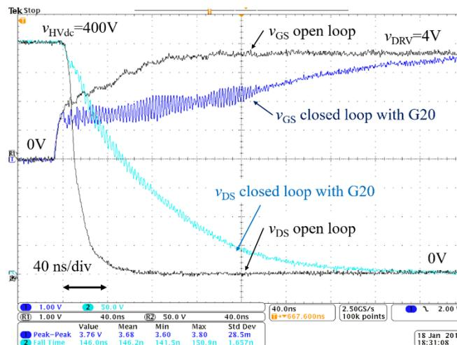
Fig. 6. Experimental results with the CMOS AGD in the 400V DC bus voltage. With the closed-loop, the  $dv/dt$  is attenuated from 45V/ns to 6.6V/ns.
