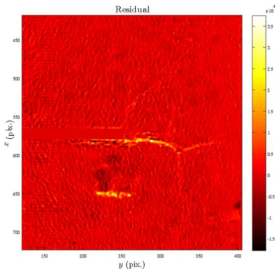
Figure 9: Experimental crack path obtained by DIC
