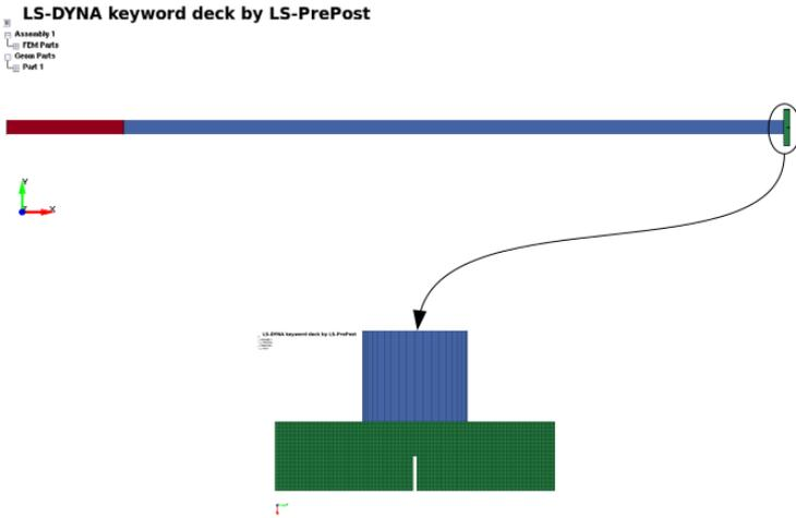
Figure 3: FE mesh of the one-point bending test: global view and zoom over the contact between the bar and the specimen
