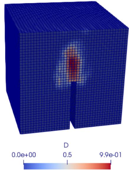
Figure 4: Damage field  $D$  obtained during the failure of the specimen
