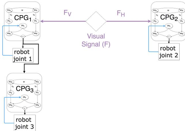
Fig. 2. CPG architecture. The shoulder pitch joint receives the vertical visual signal  $F_V$  as an input and its output is the input of the CPG controlling the elbow yaw joint; the shoulder roll joint receives the horizontal visual signal  $F_H$  as an input
