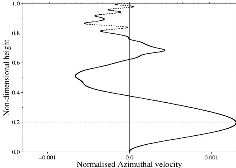
**Figure 3.** Azimuthal velocity averaged over planar annuli  $0.35r_{dom} > r > 0.3r_{dom} > r_{jet}$  as a function of height, normalised by  $\Omega r_{dom}^2 / \bar{r}$ . The location of the virtual origin is shown by a dashed line.
