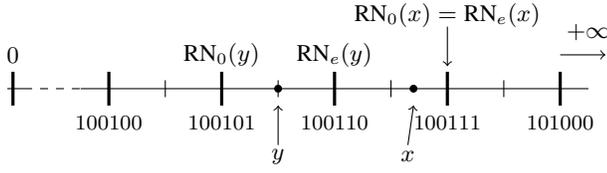
Fig. 1: Round-to-nearest ties-to-zero (assuming we are in the positive range). Number  $x$  is rounded to the (unique) FP number nearest to  $x$ . Number  $y$  is a halfway case: it is exactly halfway between two consecutive FP numbers: it is rounded to the one that has the smallest magnitude.
