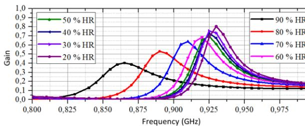
Fig. 5 Antenna gain as a function of humidity
