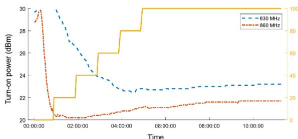
Fig. 7 Sensor temporal behavior to gas concentrations
