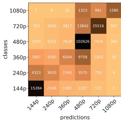
Fig. 1. Confusion matrix for kNN-based video resolution prediction.
