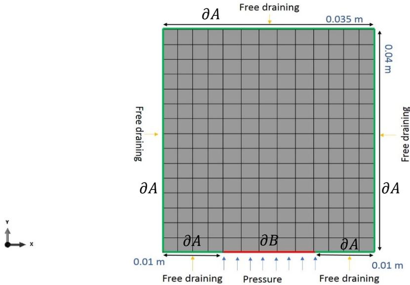
Figure 3 – The specific dimensions and boundary conditions of the numerical test are used both for the models using FEM and SGP method. The mesh size is 0.03 m (along surface  $\partial B$ ), 0.025 m and 0.0267 m (along surfaces  $\partial A$  in the horizontal and vertical directions, respectively).
