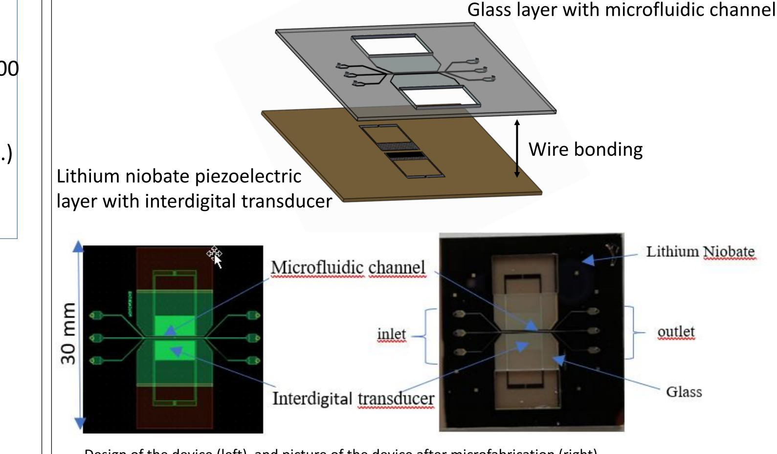
Design of the device (left), and picture of the device after microfabrication (right)
