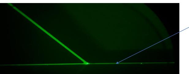
Laminar flow along the channel after injection of fluorescent beads (0,5 μm)
