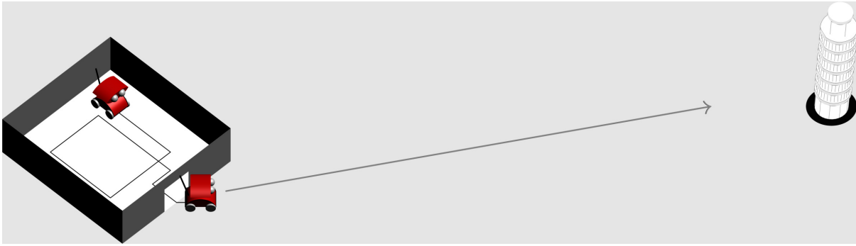
Figure 3: Numerical experiment. A robot having approximately known initial position and unknown orientation explores a room, and builds a map of 8 characteristic unknown features. Then, it leaves the building until it observes the bearing of a clearly visible landmark with known location (the Pisa tower). This new observation brings information about its orientation, and consequently on the general orientation of the map it has built.
