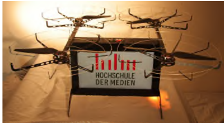
Figure 4: Indoor prototype of our DisplayDrone
