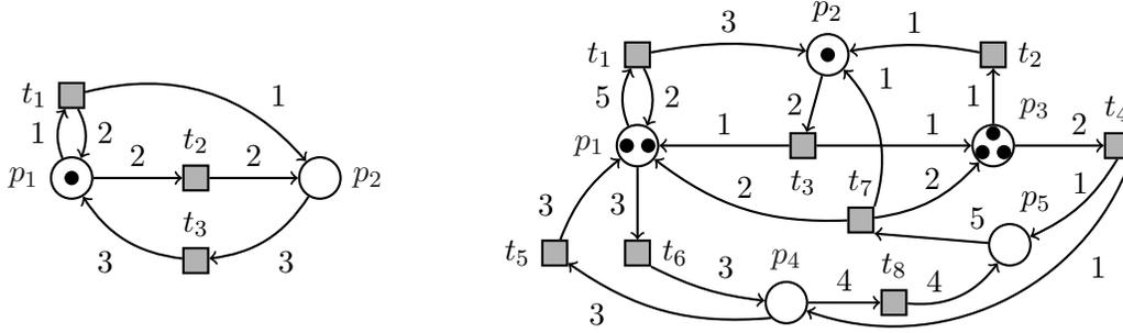
Figure 9. The live and strongly connected but unbounded JF system on the left is not m-live, since adding a token to  $p_1$  allows to fire  $t_2$ , leading to a deadlock. On the right, the JF system is strongly connected, structurally bounded (since it is  $\mathbb{1}$ -conservative), live and reversible; however, it is not m-live, since adding a token to  $p_3$  and firing two times  $t_4$  leads to a deadlock.
