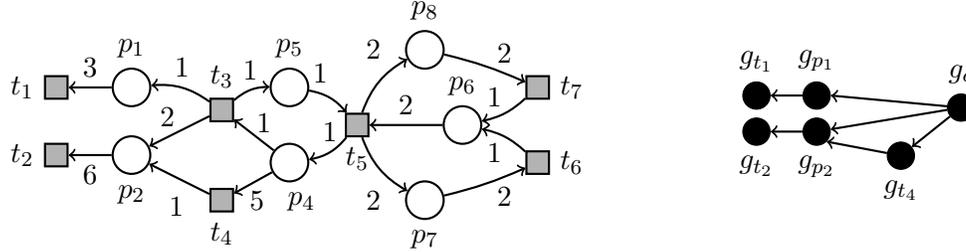
Figure 3. On the right, the reduced graph represents the net on the left. The node  $g_c$  represents the subnet  $c$  defined by places  $p_4, p_5, p_6, p_7, p_8$  and transitions  $t_3, t_5, t_6, t_7$ .
