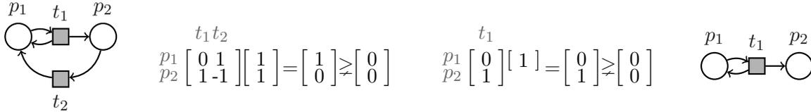
Figure 7. The strongly connected FA net on the left is sur-consistent, but is not small sur-consistent, since it contains the proper, non-empty sur-consistent T-subnet induced by  $\{t_1\}$ , which is depicted on the right. The incidence matrices of both nets show the sur-consistency of each net.
