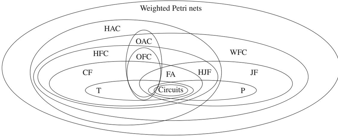
Figure 2. Some classes and subclasses of weighted systems ordered by inclusion of their structurally defined elements. A proper structural inclusion does not necessarily represent a proper expressiveness inclusion. Each class is represented by its name surrounded by an ellipse, except the Fork-Attribution (FA) class, which is represented by the intersection of the CF set with the JF set, and the HJF class, which is represented by the intersection of the HFC set with the JF set.
