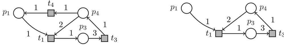
Figure 6. The net on the left is strongly connected, sub-consistent and is not JF. On the right, its unique non-empty, small, sub-consistent T-subnet, is neither strongly connected nor JF.
