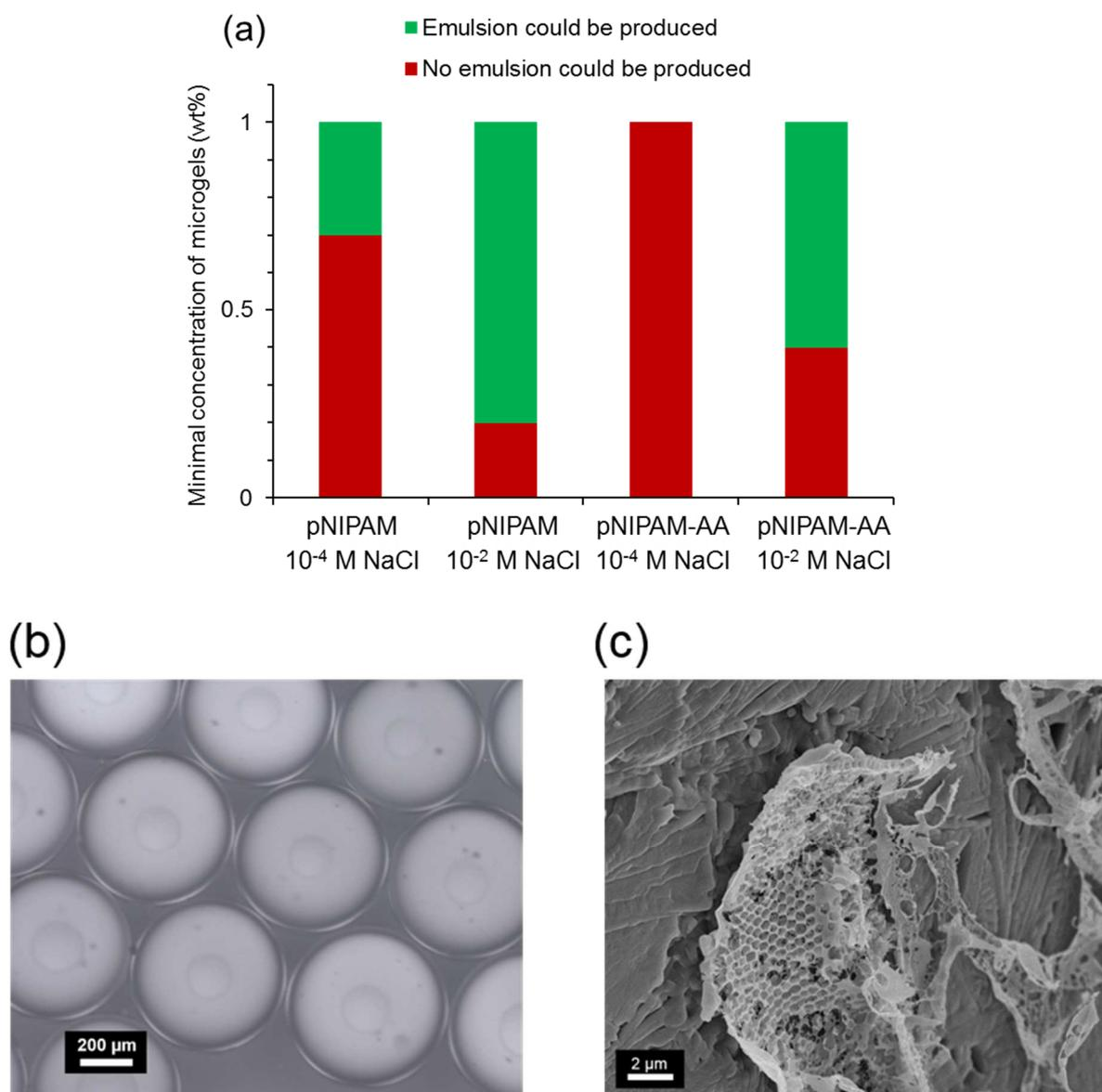
**Figure 6:** (a) Minimal microgel concentration required to produce stable drops using our microfluidic device. (b) Example of an emulsion obtained with the microfluidic device using 0.6 wt% of pNIPAM-AA with 0.1 M of NaCl. (c) CryoSEM picture obtained on an emulsion stabilized by 0.56 wt% of pNIPAM microgels with 0.05 M of NaCl.
