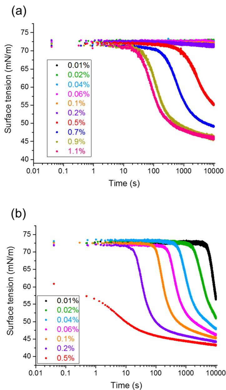
**Figure 5:** Influence of concentration and salt on the pNIPAM-AA microgels adsorption kinetics (a)  $10^{-4}$  M of NaCl and (b) and  $10^{-2}$  M.
