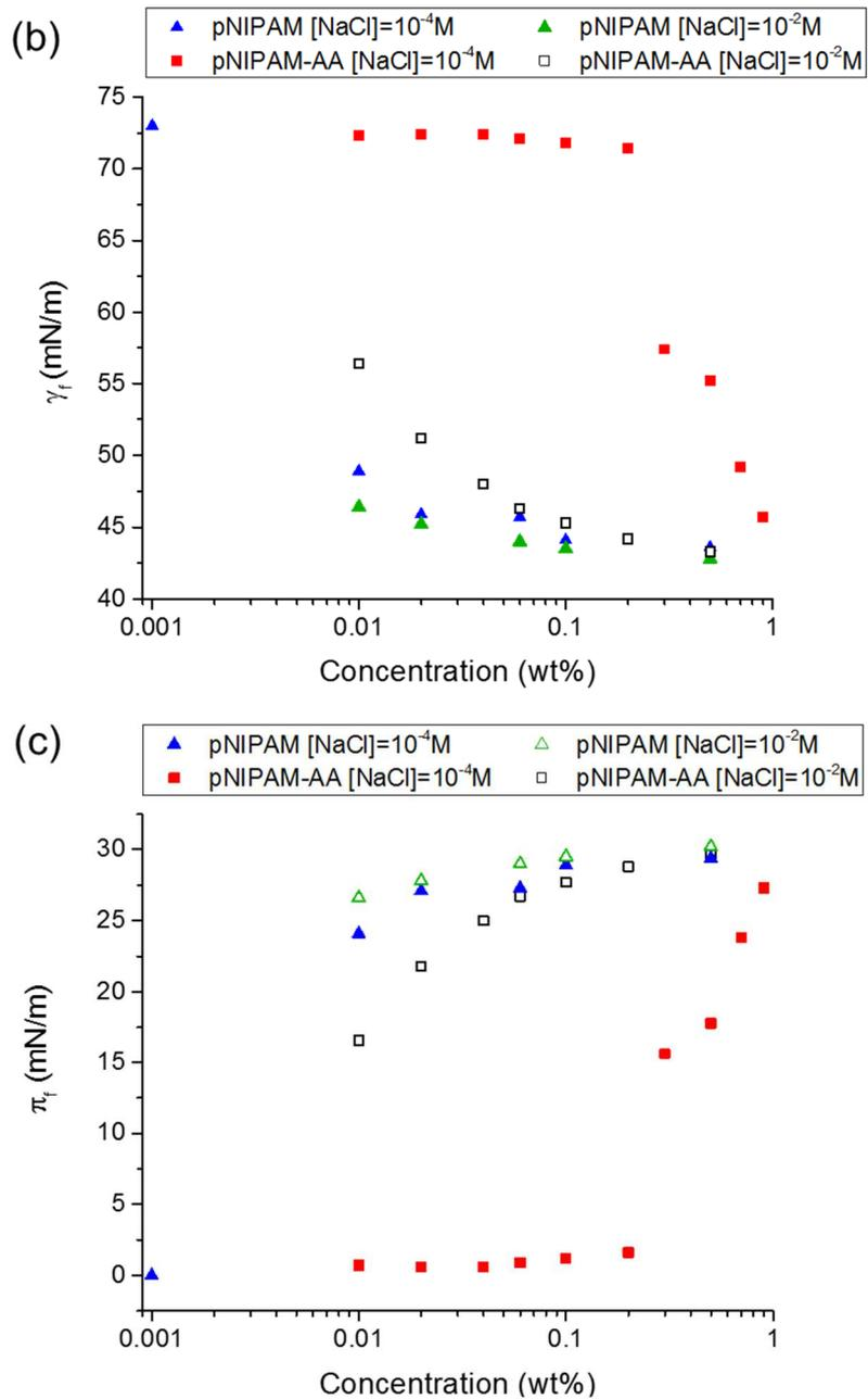
**Figure 9:** Comparison of the effect of salt and microgel concentration (a) on the adsorption kinetics assessed by  $t^*$  and on the final state through (b)  $\gamma_f$  and (c)  $\pi_f$  for neutral and charged microgels. PNIPAM microgels with NaCl =  $10^{-4}$  M (solid blue triangles), PNIPAM-AA microgels with NaCl =  $10^{-4}$  M (solid red squares), PNIPAM microgels with NaCl =  $10^{-2}$  M (open green triangles) and PNIPAM-AA microgels with NaCl =  $10^{-2}$  M (open black squares).
