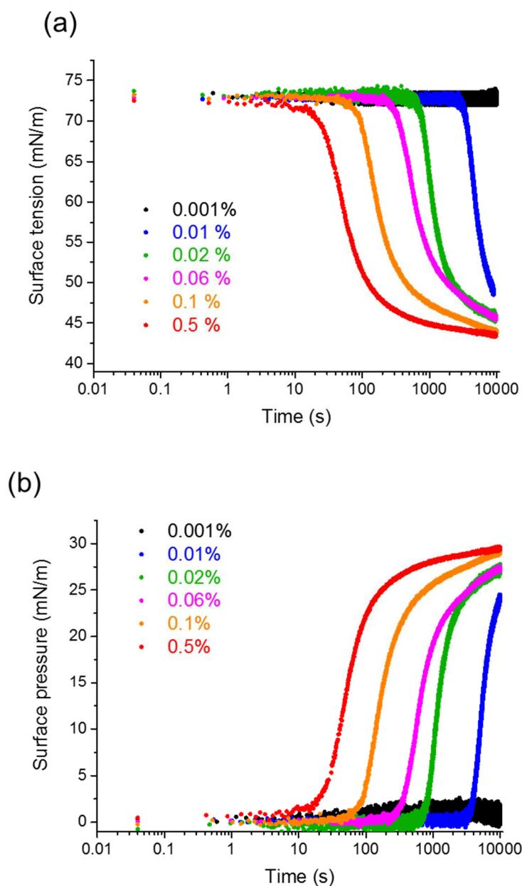
**Figure 2:** Influence of the microgels concentration on (a) the surface tension and (b) deduced spontaneous surface pressure for pNIPAM microgels with a fixed cross-linking density (BIS 2.5 mol%) in presence of NaCl at  $10^{-4}$  M.
