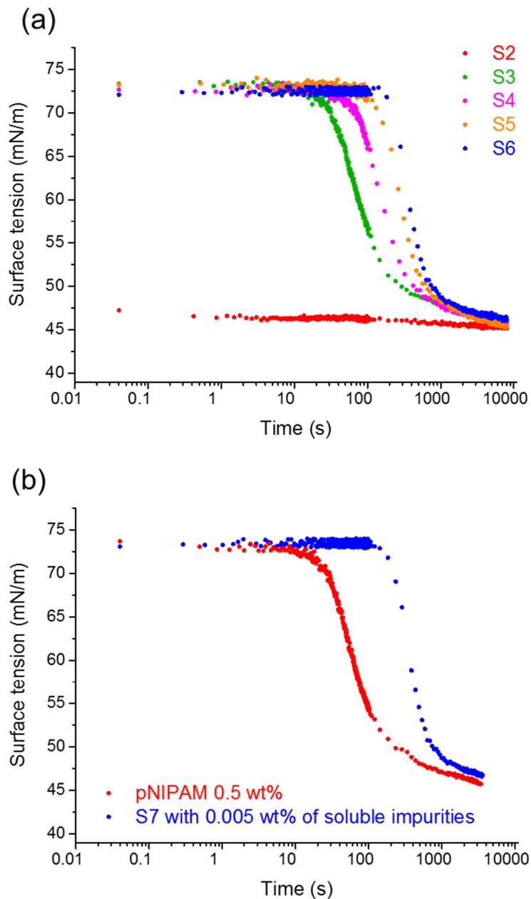
**Figure 1:** Surface properties of the various supernatants (a) kinetics of adsorption (S2: red, S3: green, S4: pink, S5: orange, S6: blue) and (b) comparison with cleaned microgels (5 cleaning steps), see text for more explanation.
