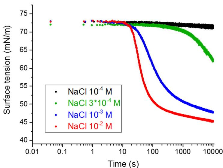
**Figure 10:** Progressive acceleration of pNIPAM-AA adsorption in presence of increasing amount of NaCl i.e. decreasing Debye lengths  $\kappa^{-1}$ .  $10^{-4}$  M NaCl  $\kappa^{-1}=30$  nm (black curve),  $3 \cdot 10^{-4}$  M NaCl  $\kappa^{-1}=17.3$  nm (green curve),  $10^{-3}$  M NaCl  $\kappa^{-1}=9.5$  nm (blue curve) and  $10^{-2}$  M NaCl  $\kappa^{-1}=3$  nm (red curve).
