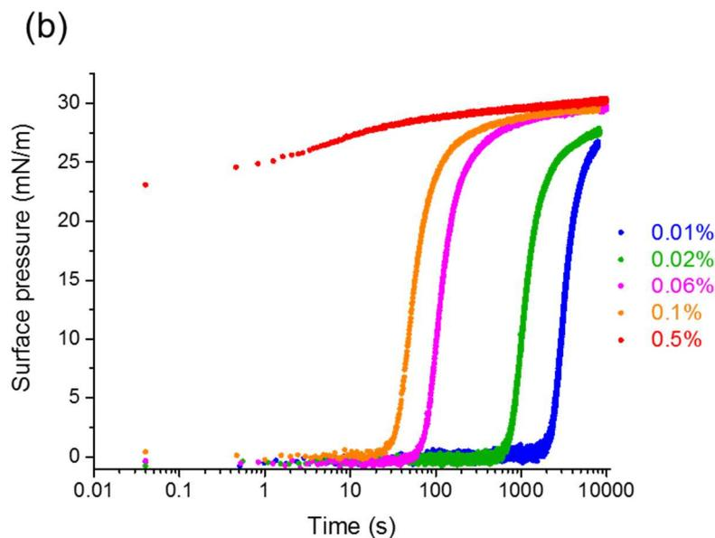
**Figure 3:** Influence of the microgels concentration on (a) the surface tension and (b) deduced spontaneous surface pressure for pNIPAM microgels with a fixed cross-linking density (BIS 2.5 mol%) in presence of NaCl at  $10^{-2}$  M.
