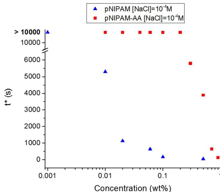
**Figure 8:** Evolution of the characteristic time  $t^*$  (corresponding to the time for  $\gamma \approx 60$  mN/m) as a function of the microgels concentration for neutral pNIPAM (blue triangles) microgels and charged pNIPAM-AA (red squares) microgels with  $[\text{NaCl}] = 10^{-4}$  M.
