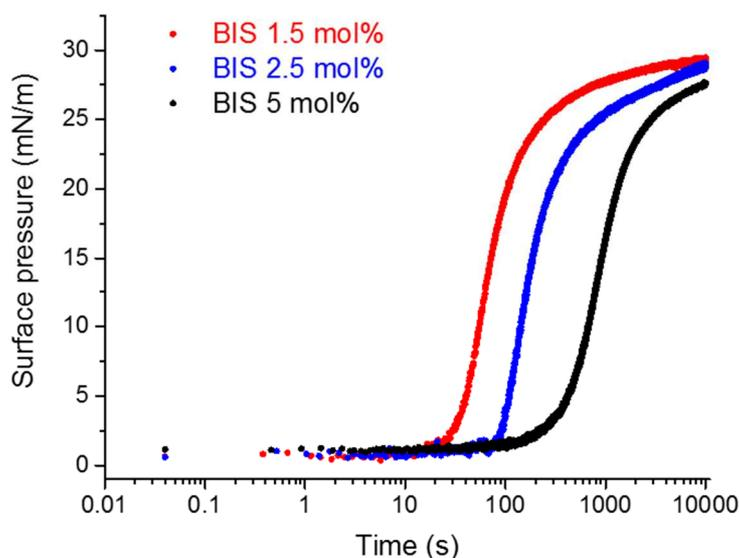
**Figure 4:** Influence of the cross-linking density on the spontaneous surface pressure. The microgel concentration is kept constant  $C_{\text{microgels}} = 0.1 \text{ wt\%}$  and the cross-linking density is varied through the BIS content: 1.5 mol% (red), 2.5 mol% (blue) and 5 mol% (black), in presence of NaCl at  $10^{-4} \text{ M}$ .
