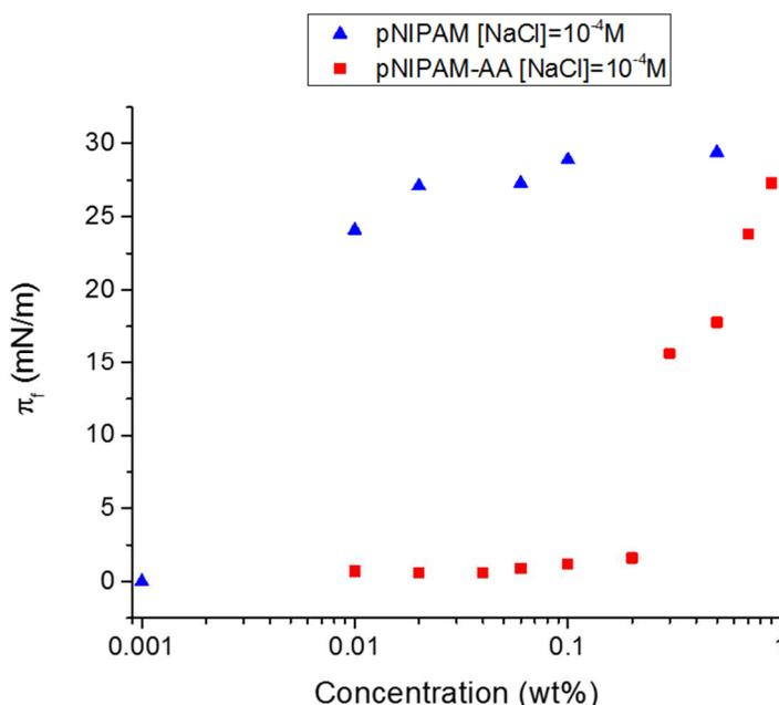
**Figure 7:** Evolution of the final spontaneous surface pressure  $\pi_f$  (at 10 000 s) as a function of the microgels concentration for “neutral” pNIPAM microgels (blue triangles) and charged pNIPAM-AA microgels (red squares) with  $[\text{NaCl}] = 10^{-4}$  M.
