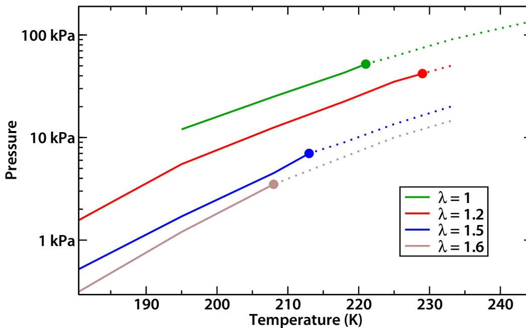
**Figure 6.** Pressure–temperature phase diagram for CO<sub>2</sub> confined in IRMOF-1, with MOF-CO<sub>2</sub> interactions multiplied by a factor of  $\lambda$  in order to understand the consequences of a modification of the chemical nature of the internal surface of the material, with fixed pore size, geometry and topology.
