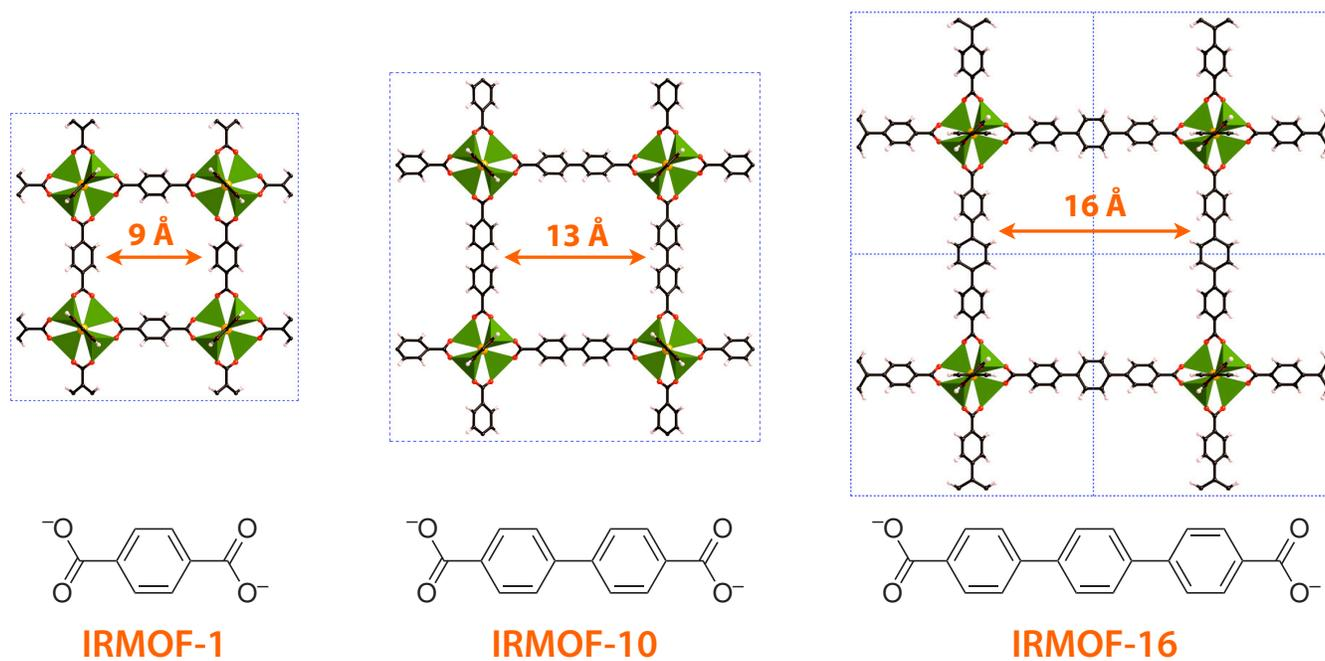
**Figure 1.** Representation of the IRMOFs studied in the present work: IRMOF-1, IRMOF-10 and IRMOF-16: unit cells, pore size and linker. For IRMOF-16, a 2×2×2 supercell is depicted.
