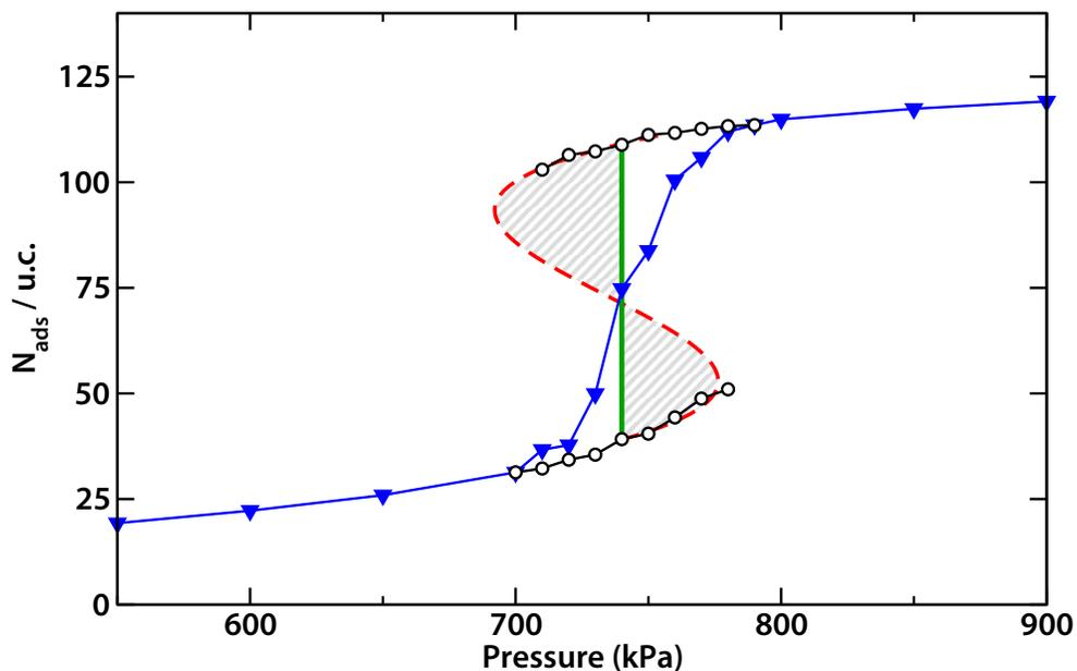
**Figure 4.** First-order phase transition of CO<sub>2</sub> adsorption in IRMOF-16 at 250 K. Blue triangles correspond to averages from GCMC simulations. Open circles represent individual “empty” and “filled” phases observed in the GCMC simulations in the 700–800 kPa range. The thermodynamic equilibrium pressure is indicated by the vertical green line, and the spinodal (calculated as a third-power best fit complying with Maxwell’s rule) is indicated in dashed red.
