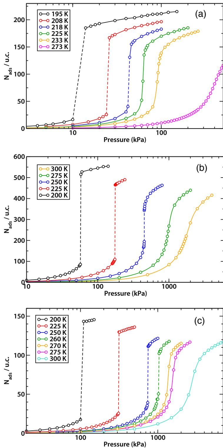
**Figure 2.** CO<sub>2</sub> adsorption isotherms in IRMOF-1 (a), IRMOF-10 (b) and IRMOF-16 (c) in the 195–300 K range of temperature. Each symbol corresponds to a single  $(\mu, V, T)$  GCMC simulation. Lines are added to guide the eye. Vertical dashed lines correspond to first-order phase transitions.
