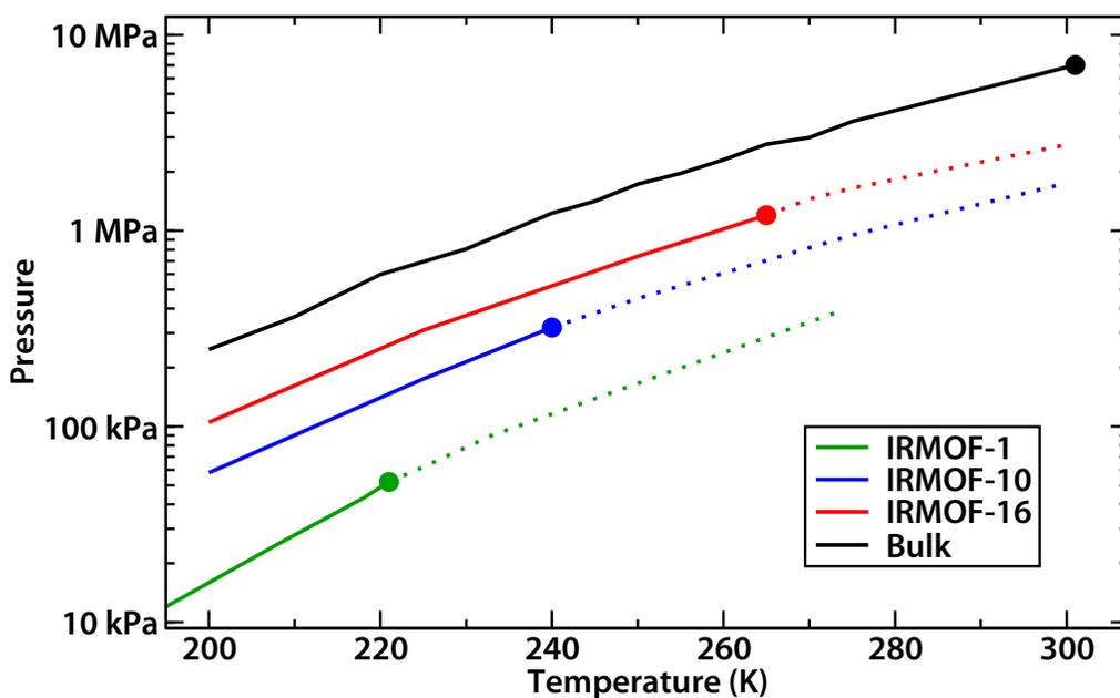
**Figure 3.** Pressure–temperature phase diagram for CO<sub>2</sub> confined in IRMOF-1, -10 and -16, compared to the bulk phase. Solid lines represent liquid-vapor first-order phase transitions, filled circles indicate critical points and dotted lines indicate continuous adsorption transitions.
