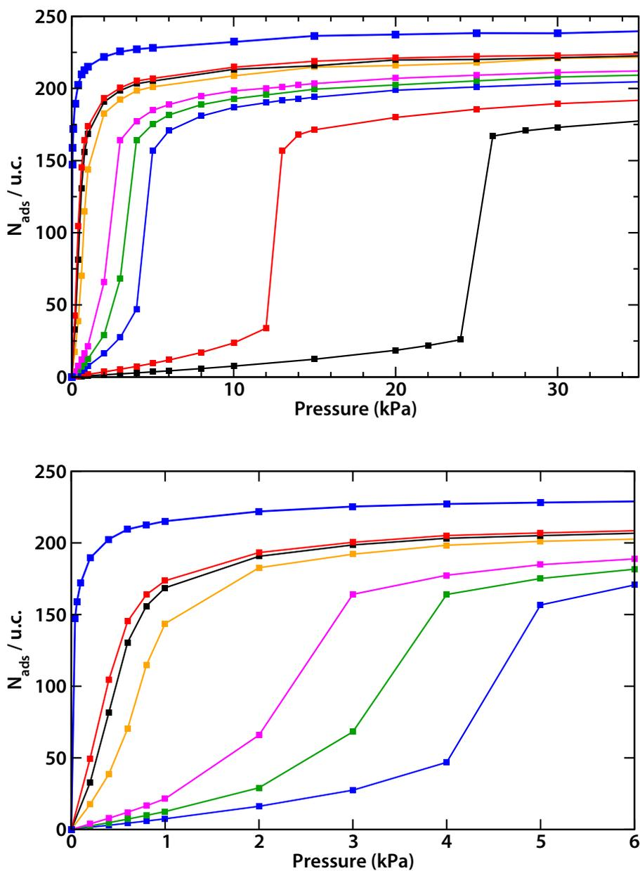
**Figure 5.** CO<sub>2</sub> adsorption isotherms in IRMOF-1 at 208 K with scaled CO<sub>2</sub>–IRMOF interactions, for different values of the scaling parameter  $\lambda$ : 1 (black), 1.2 (red), 1.5 (blue), 1.6 (green), 1.7 (pink), 2.0 (orange), 2.5 (black), 2.7 (red) and 3.0 (blue). Lower panel displays a zoom of the low-pressure range (up to 6 kPa).
