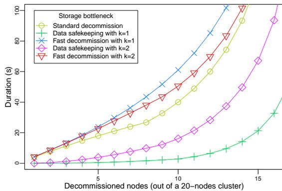
Fig. 9. Lower bounds for the duration of the data-safekeeping phase and fast decommission compared with the lower bound for the standard decommission in case of a storage bottleneck for  $k = 1$  and  $k = 2$ . Each node initially hosts 50 GiB of data, and the reading and writing speed of the storage is set to 1.25 GiB/s.
