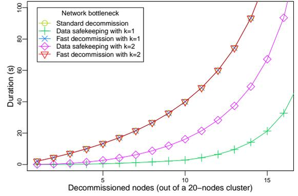
Fig. 8. Lower bounds for the duration of the data-safekeeping phase and fast decommission compared with the lower bound for the standard decommission in case of a network bottleneck for  $k = 1$  and  $k = 2$ . Each node initially hosts 50 GiB of data, and the network bandwidth is set to 1.25 GiB/s.
