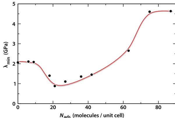
**Figure 4.** Change in the elastic response of the ZIF *nog*<sup>45</sup> as a function of the number of methane molecules adsorbed species, obtained from isostress-isothermal MD simulations at 300 K.<sup>32</sup> The ordinate is the smallest elastic modulus of the material, i.e. the lowest eigenvalue  $\lambda_{\min}$  of the elastic stiffness tensor. Uncertainty on each value is of the order of 0.1 GPa (see ref. 32).
