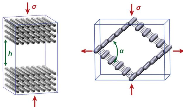
**Figure 1:** Sketch of the two model microporous frameworks. Left: slit-pore; right: lozenge-shaped pore. The red arrows represent the direction of the stress exerted on the solid frameworks, and the unique order parameters of the deformation are represented in green.
