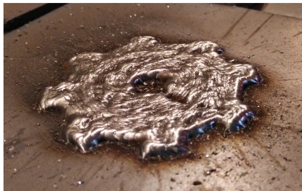
Figure 10. The result of printed gear (60 mm diameter) with 2 mm layer height.
