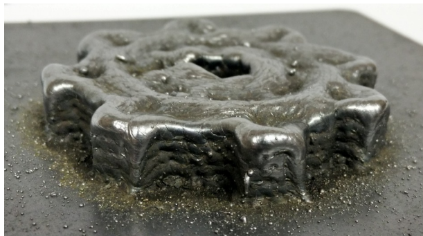
Figure 15. The finished 3-D printed gear (60 mm diameter) (5 layers).
