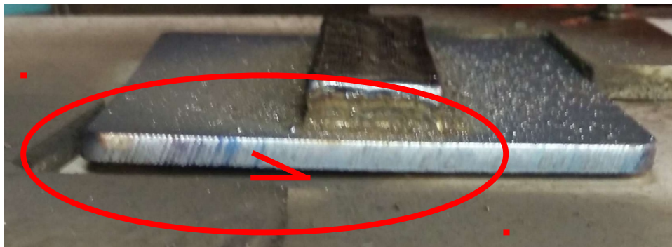
Figure 18. Thermal induced substrate deformation which is indicated by the angle symbol (101.6 mm × 31.75 mm). When corrected the substrate remains flat.
