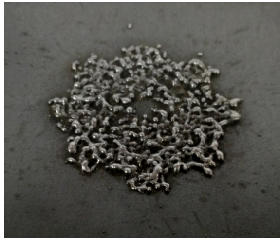
Figure 9. The result of printed gear (60 mm diameter) with 1 mm layer height.
