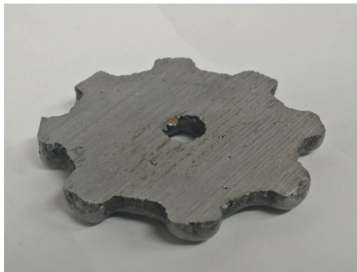
Figure 15. The finished 3-D printed gear (60 mm diameter) (5 layers).
