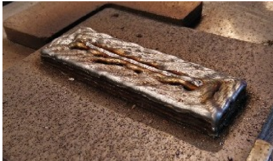
Figure 11. Poor surface quality after third layer of printing speed 10 mm/s on block (101.6 mm × 31.75 mm).
