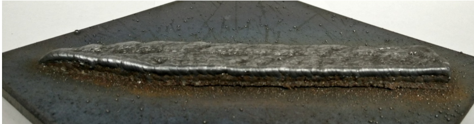
Figure 13. 3 layers of 3-D printed chisel (140 mm × 20 mm × 20 mm).
