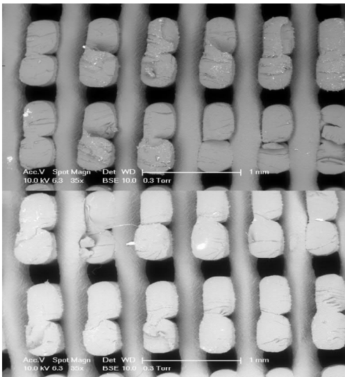
Figure 9: The surface of the fracture interface of 1 hour annealed (top) and unannealed (bottom) samples, taken with an Environmental Electron Scanning Microscope (ESEM).
