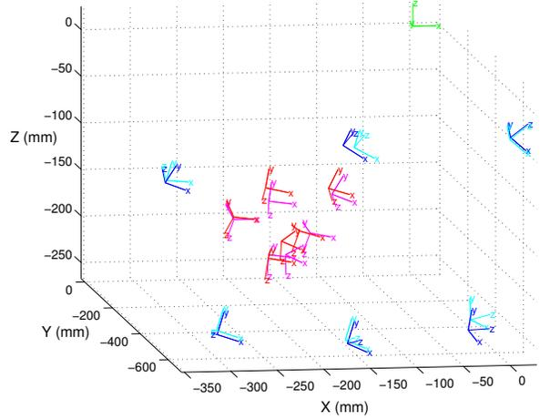
Fig. 7. Frames of the arm ( $\mathbf{R}_{s1}$ ) without (red) and with robot (magenta). Frames of the forearm ( $\mathbf{R}_{s2}$ ) without (blue) and with robot (cyan). The green frame stand for the global frame origin  $\mathbf{R}_r$ .
