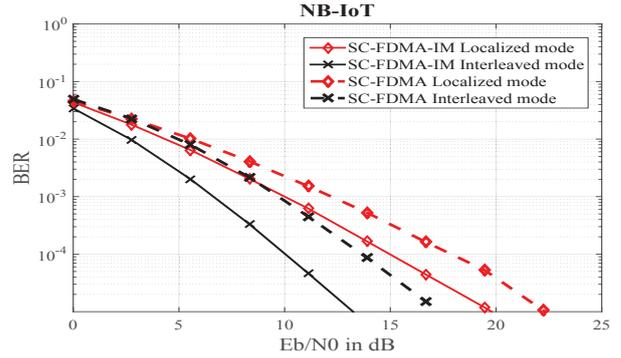
Fig. 5. BER performance for SC-FDMA-IM in NB-IoT scenario
