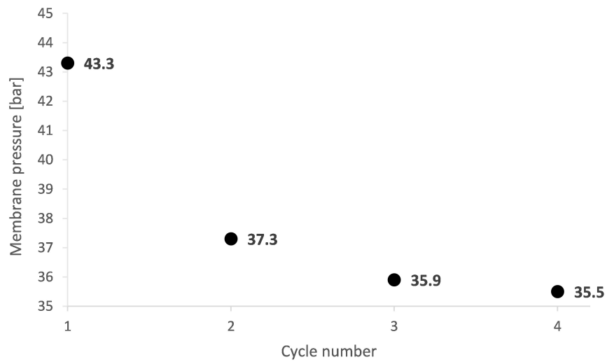
Figure 14: Effect of cycle number on membrane pressure at a composition of 10% water, 5% surfactant and 85% Marcol 82 at a flowrate of 50 mL/min
