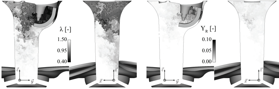
Fig. 7: Plane cut normal to the x axis (left), y axis (right) intersecting the ducts by their axis at -10.5\text{ CAD} coloured by the air fuel equivalence ratio \lambda with an iso-contour of stoichiometric equivalence ratio (—).
