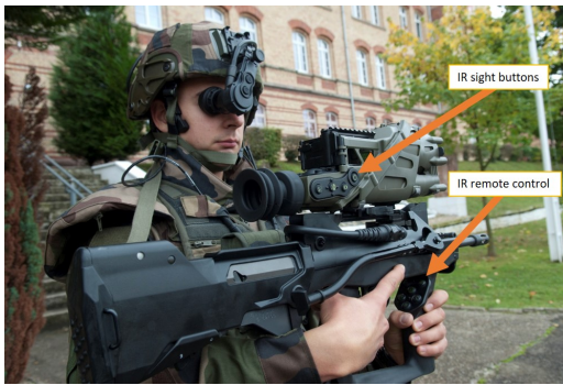
Figure 1: FELIN soldier equipped with the IR sight on the FAMAS rifle [3]
