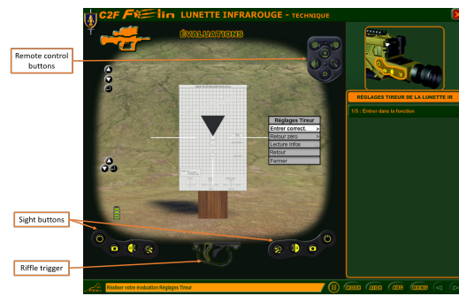
Figure 3: Sight calibration training module on the EAO FELIN software
