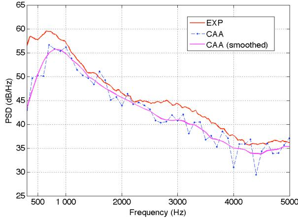
Figure 20. Predicted and measured 3D spectra (dB/Hz)
