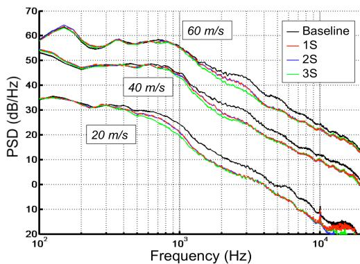
Figure 4. Baseline and ONERA wing spectra ( $90^\circ$ )
