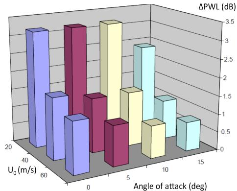
Figure 5. PWL reductions (dB) using 3S wing
