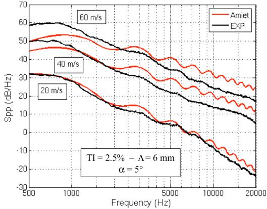
Figure 12. Predicted and measured PSD at 90°
