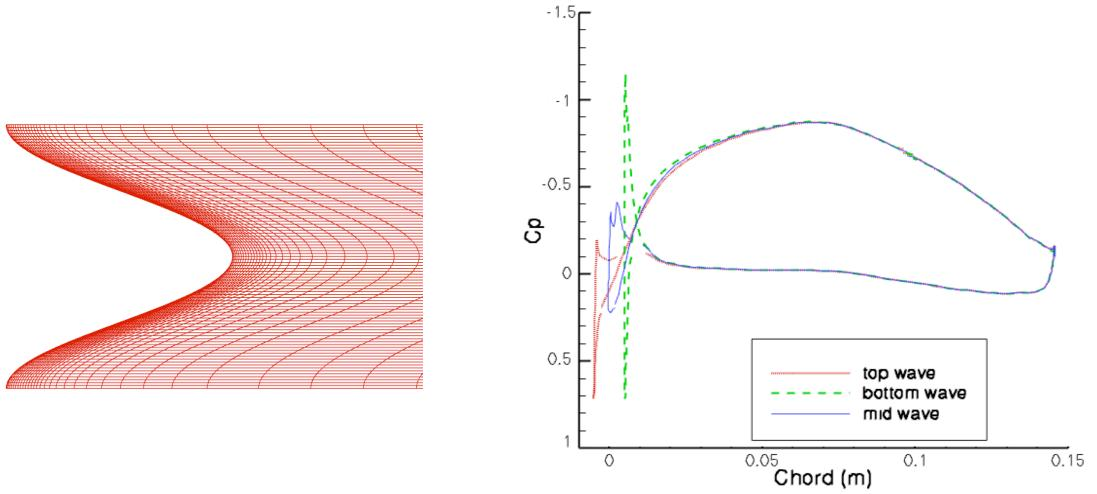
Figure 9. 3D RANS wavy-edge mesh (left) and computed  $C_p$  distributions ( $U_0 = 60$  m/s,  $\alpha = 0^\circ$ )
