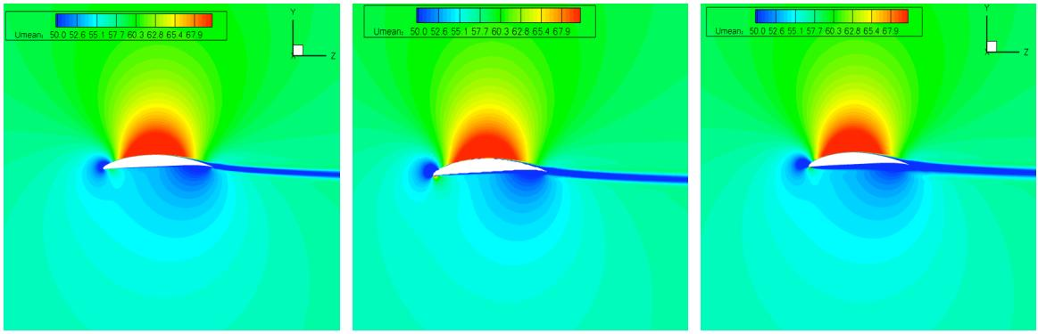
Figure 10. Spanwise cuts of RANS mean flow velocity field around 2S and baseline wings:
