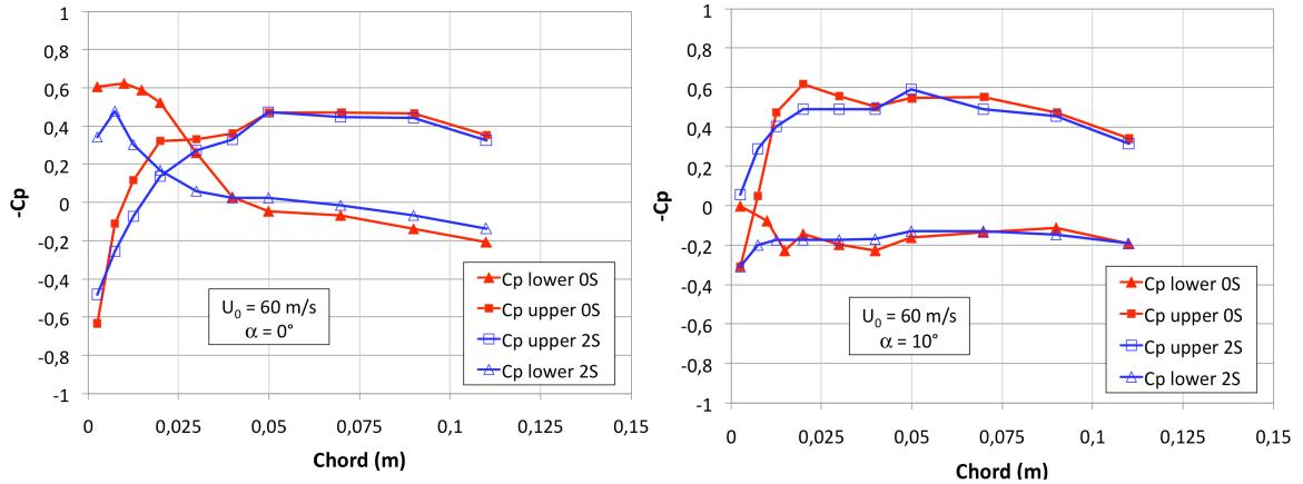
Figure 8.  $C_p$  distributions for baseline and ONERA 2S wing measured at  $\alpha = 0^\circ$  (left) and  $\alpha = 10^\circ$  (right)
