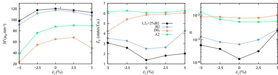
FIG. 1. Impact of the tetragonal distortion on the properties of the 4 phases of  $\text{Co}_2\text{MnSi}$ : a) on the magnetization  $M$ , b) on the total density of states at the Fermi level  $Z_F$  and c) on the Gilbert damping parameter  $\alpha$ .
