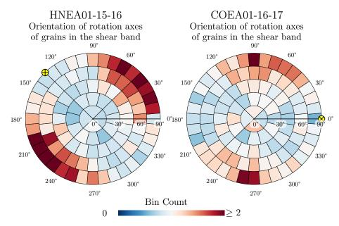
Figure 10: Comparison of the rotation axes for the grains in the shear band in specimens HNEA01 and COEA01. The yellow dot indicates the orientation of the *direction of maximum* slope in the shear band
