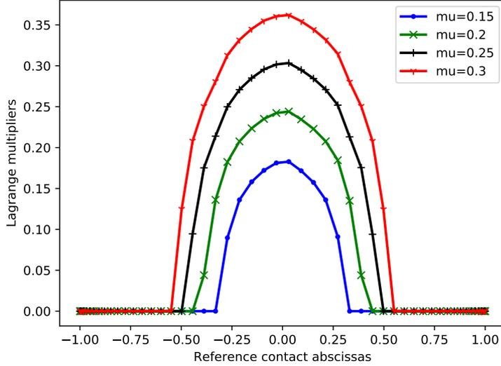
Figure 4: Test case (a) - Lagrange multipliers obtained with the collocation method as a function of the abscissas in the reference configuration for the parameter values  $\mu \in \{0.15, 0.2, 0.25, 0.3\}$ . Vanishing values correspond to nodes where the contact between the two disks is not established at equilibrium.
