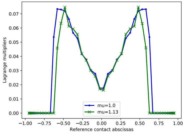
Figure 18: Test case (c) - Lagrange multipliers as a function of the abscissas in the reference configuration for the parameters  $\mu \in \{1.0, 1.13\}$ . Vanishing values correspond to nodes where the contact between the ring and the rectangular surface is not established at equilibrium.
