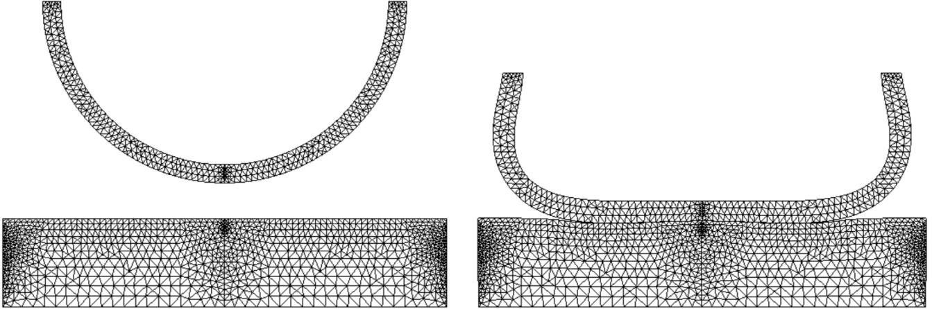
Figure 17: Test case (c) - Left: Reference domain  $\Omega$  with  $R_1 = 1\text{m}$  and mesh with  $\mathcal{N} = 1590$  nodes. Right: Deformed configuration resulting from the HF displacement field  $u_N(\mu)$  for  $R_1 = 1\text{m}$ .
