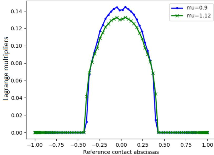
Figure 6: Test case (b) - HF Lagrange multipliers obtained with the collocation method for the parameter values  $\mu \in \{0.9, 1.12\}$ . Vanishing values correspond to nodes where the contact between the two half-disks is not established at equilibrium.
