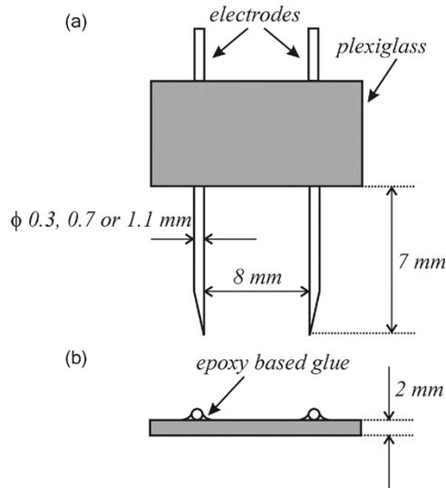
FIGURE 3. Experimental set-up for electroporation measurements as performed by Sel *et al.* 3 electrodes diameter are considered. The piece of rabbit liver is located below the plexiglass on a thickness of 7 mm [19].
