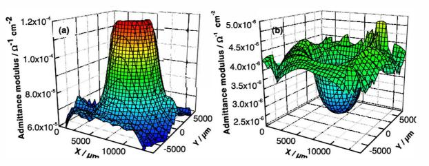
Fig. 8. Mappings obtained at 10 Hz above the Al/Cu couple: (a) after 2 h of immersion in a 10<sup>-3</sup> M NaCl solution and (b) after 20 h of immersion in deionised water (without NaCl) containing 8-HQ+BTA; static electrode.
