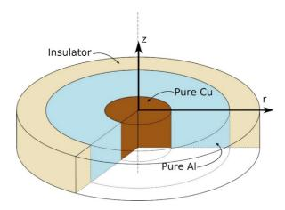
**Fig. 1.** Schematic representation of the pure aluminium/pure copper model couple. The radii of the two cylinders were equal to 1 and 0.315 cm for aluminium and copper bars, respectively. The electrode was then embedded in an epoxy resin so that a disk electrode was obtained at the extremity.
