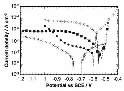
Fig. 3. Polarization curves obtained on AA2024 after 20 h of immersion in a 0.1 M Na<sub>2</sub>SO<sub>4</sub> + 0.05 M NaCl solution: () without inhibitor; () with BTA; () with 8-HQ and (x) with 8-HQ + BTA; electrode rotation rate: 500 rpm.
