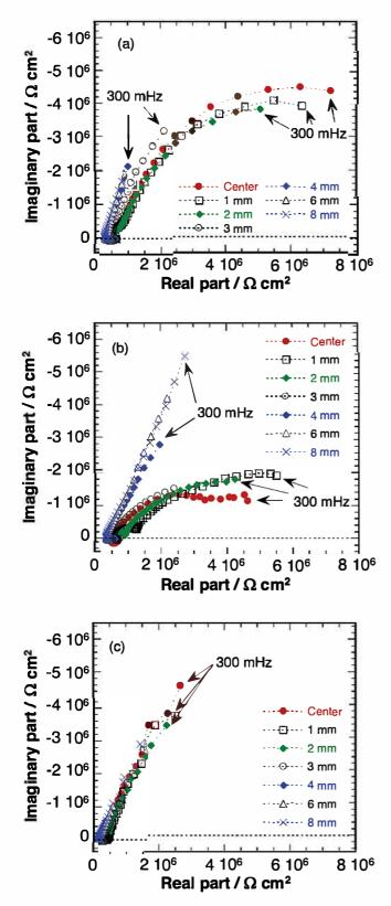
Fig. 9. Local impedance spectra obtained for different radial positions above the Al/Cu couple after 20 h of immersion in aqueous solution (deionised water without NaCl): (a) with BTA, (b) with 8-HQ and (c) with 8-HQ +BTA; static electrode.
