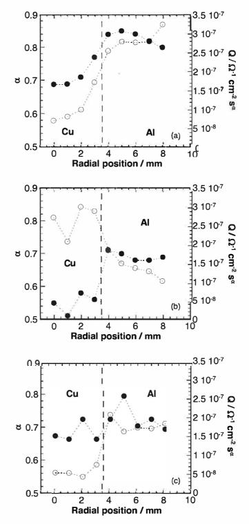
Fig. 10. (•)  $\alpha$  and (O) Q parameters obtained from the local impedance spectra for different radial positions above the Al/Cu couple after 20 h of immersion in aqueous solution (deionised water without NaCl): (a) with BTA, (b) with 8-HQ and (c) with 8-HQ+BTA.
