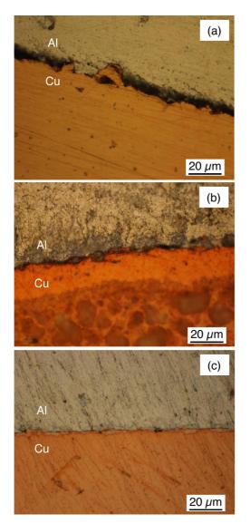
**Fig. 11.** Optical micrographs of the Al/Cu couple interface after 20 h of immersion in an aqueous solution (deionised water without NaCl): (a) with BTA, (b) with 8-HQ and (c) with 8-HQ+BTA; static electrode.
