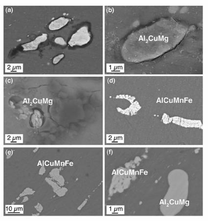
Fig. 4. SEM micrographs of AA2024 surface after 20h of immersion in a 0.1 M Na<sub>2</sub>SO<sub>4</sub> + 0.05 M NaCl solution containing: (a) and (b) BTA, (c) and (d) 8-HQ and (e) and (f) 8-HQ + BTA; electrode rotation rate: 500 rpm.
