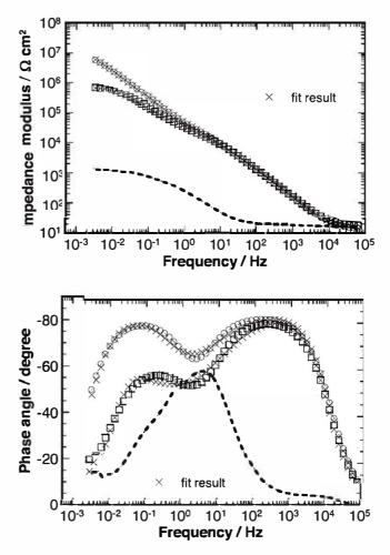
Fig. 7. Electrochemical impedance diagrams obtained on AA2024 after 20 h of immersion at  $E_{corr}$  in a 0.1 M Na<sub>2</sub>SO<sub>4</sub> + 0.05 M NaCl solution containing: ( $\Box$ ) 8-HQ and ( $\bigcirc$ ) 8-HQ + BTA. The diagram obtained in the absence of inhibitor is reported in dotted line for comparison; electrode rotation rate: 500 rpm.
