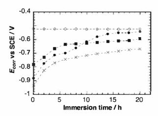
Fig. 2. Corrosion potential ( $E_{corr}$ ) of AA2024 as a function of time in a 0.1M Na<sub>2</sub>SO<sub>4</sub> + 0.05 M NaCl solution: ( $\bigcirc$ ) without inhibitor; ( $\blacksquare$ ) with BTA; ( $\spadesuit$ ) with 8-HQ and ( $\times$ ) with 8-HQ + BTA; electrode rotation rate: 500 rpm.
