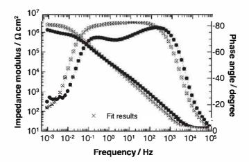
Fig. 5. Electrochemical impedance diagrams obtained on pure aluminium after 20 h of immersion at  $E_{corr}$  in a 0.1 M Na<sub>2</sub>SO<sub>4</sub> + 0.05 M NaCl solution: ( $\bigcirc$ ) without inhibitor and ( $\bullet$ ) with 8-HQ; electrode rotation rate: 500 rpm
