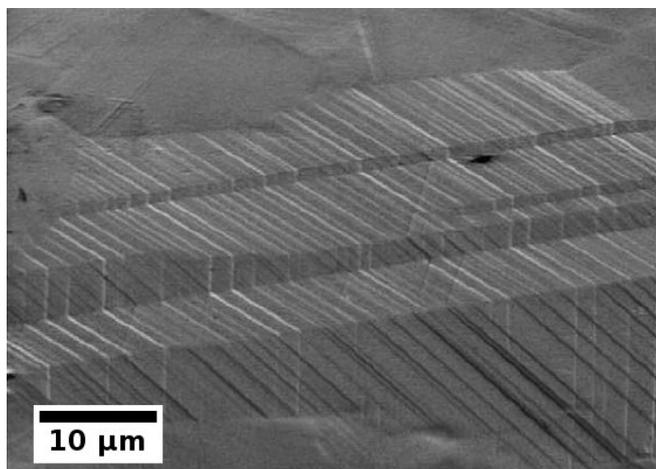
*Figure 3.6 - Typical cross twinning at the surface of the polished test sample.*
