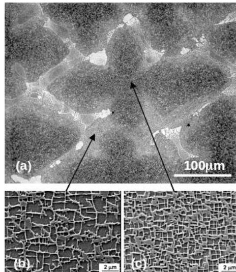
Figure 2.2 - Dendritic microstructure of the as-cast MC-NG SC superalloy normal to the  $\langle 001 \rangle$  growth direction: (a) at the dendrite scale, imaged by light microscopy (LM); (b) and (c)  $\gamma'$  precipitates, imaged by scanning electron microscopy (SEM).
