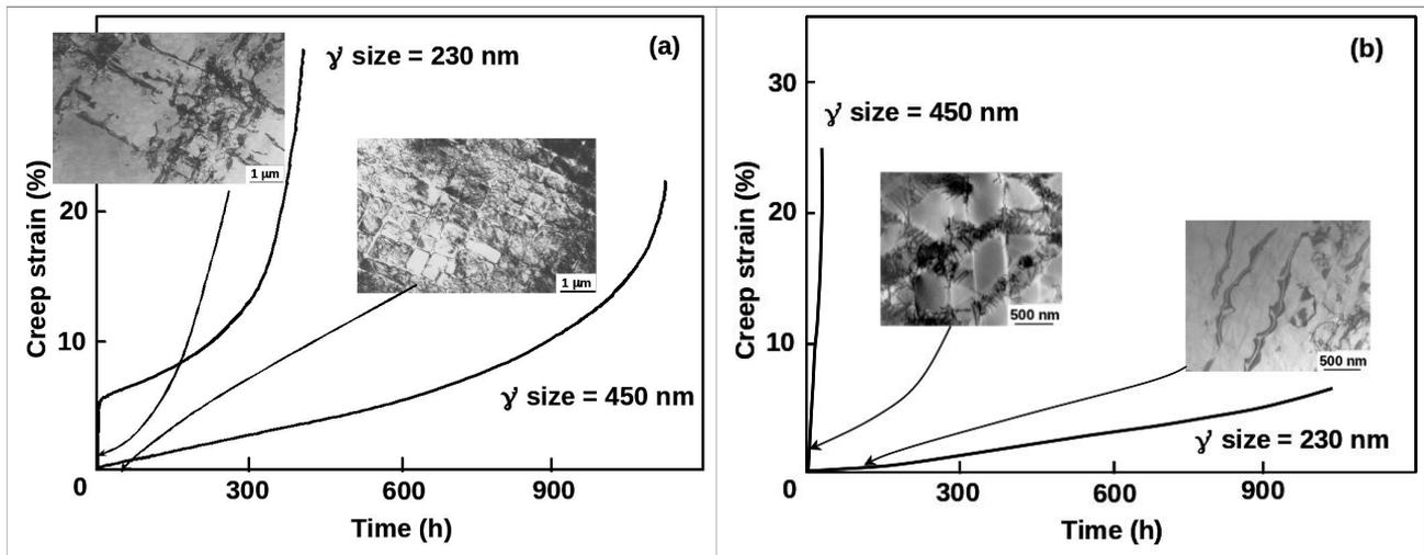
Figure 2.4 - Effect of the  $\gamma'$  precipitate size on the deformation mechanisms and creep behaviour at 760°C and 750 MPa of CMSX-2 SC superalloy along: a)  $\langle 001 \rangle$ ; b)  $\langle 111 \rangle$ .
