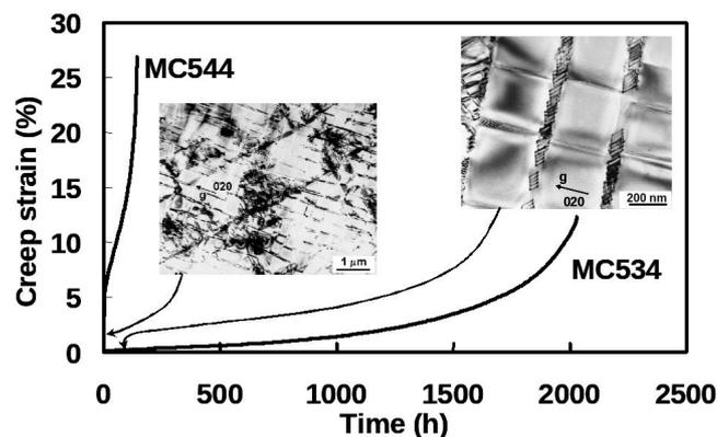
Figure 2.5 - Creep behaviour and deformation mechanisms at 760°C and 840 MPa of MC544 and MC534 <001> single crystal specimens.
